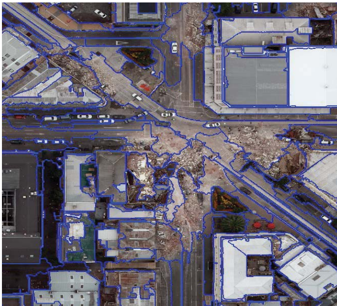
Figure 4.2.1-1 Example of good segmentation showing good coverage of visually recognizable objects by segmented image objects 2
