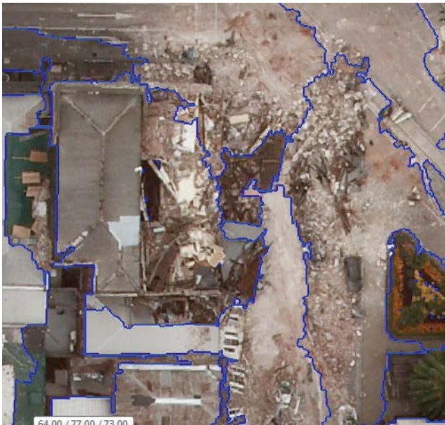
Figure 4.2.1-3 Example of poor segmentation results showing too large of an image object for the visually recognizable objects. 3
