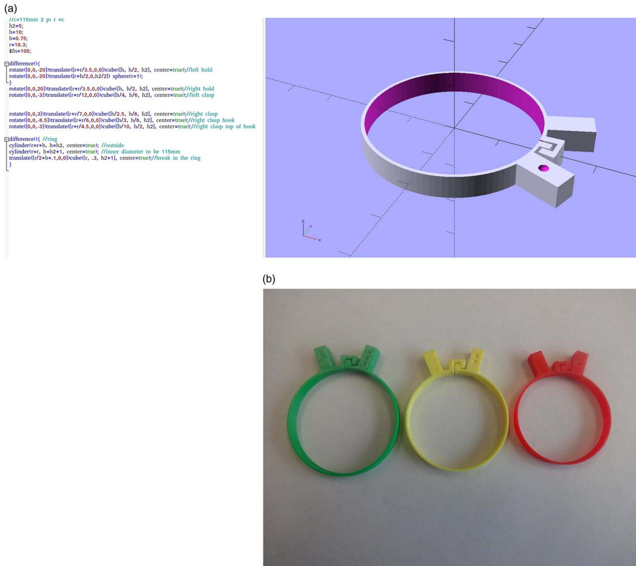
**Fig. 1** (a) The OpenSCAD code (left) and solid model (right) of the 115 mm 3-D printable click-MUAC band<sup>(24)</sup>. (b) Colour-coded 3-D printed click-MUAC bands. From left to right the bands have an inner circumference of 135 mm (green; three dimples), 125 mm (yellow; two dimples) and 115 mm (red; one dimple). (3-D, three dimensional; MUAC, mid-upper arm circumference)
