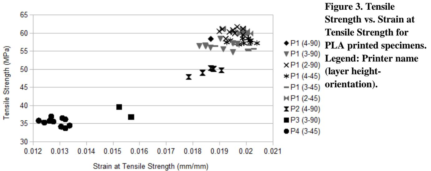
**Figure 3. Tensile Strength vs. Strain at Tensile Strength for PLA printed specimens. Legend: Printer name (layer height-orientation).**
