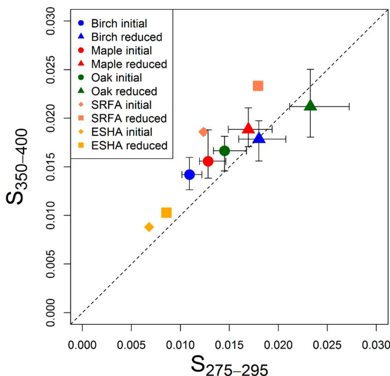
**Figure 2.** Mean absorption indices,  $S_{275-295}$  and  $S_{350-400}$ , for leaf litter leachates. Borohydride treatment (reduced) causes increases in both metrics for all samples. Both spectral slopes do not appear to distinguish leaf leachates from HA and FA standards. Error bars indicate range of values for all four time points of each species. Dashed line indicates a spectral ratio of 1.
