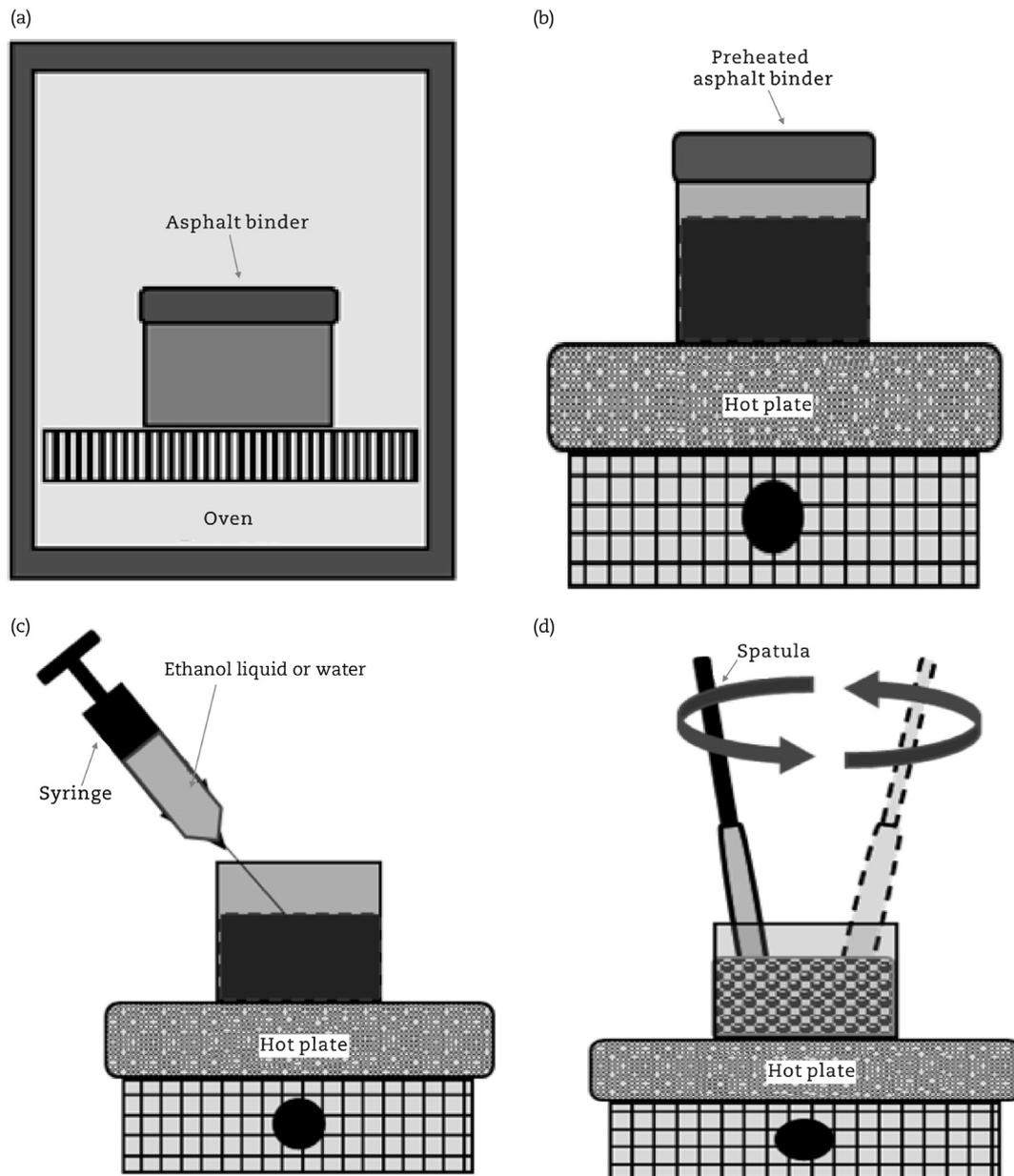
**Fig. 1 – Preparation of the foamed asphalt. (a) Preheat the asphalt binder that was initially poured into a small container in an oven at the test temperature. (b) Place the container with asphalt binder on a preheated hot plate. (c) Add in specified amount of foaming agent (ethanol or water). (d) Stir the binder and the foaming agent(s) for about 30 s before recording the temperature.**
