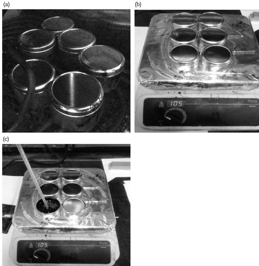
**Fig. 2 – Test procedure. (a) Asphalt binder preheated in an oven for at least 90 min at foaming temperature. (b) The container placed on a hot plate to avoid temperature reduction due to room temperature. (c) Measurement of temperature after binder foaming process.**
