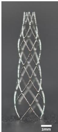
Fig. 6. Patient-specific NiTi stent produced with LPBF.
