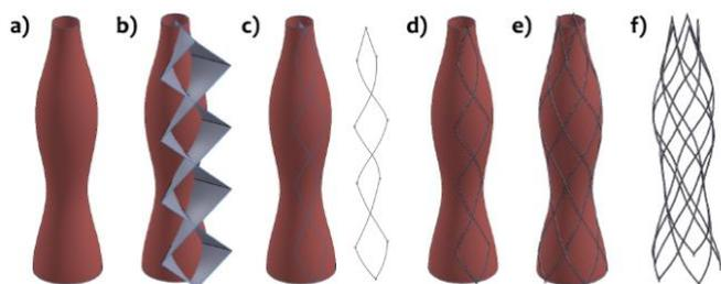
Fig. 2. (a) Base surface from mimicked patient data, (b) reference surfaces for the mesh, (c) baseline obtained from the intersection between the base surface and reference (d) 3D wireframe with circular profile following the base surface, (e) complete stent on the base surface, (f) final stent.
