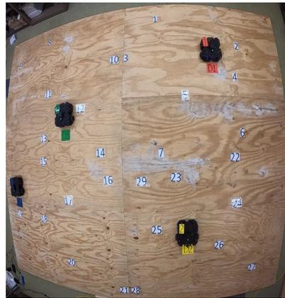
**Figure 4.** An experimental scene for one of the field experiments. The colored locations represent the depots, and others represent the target locations.
