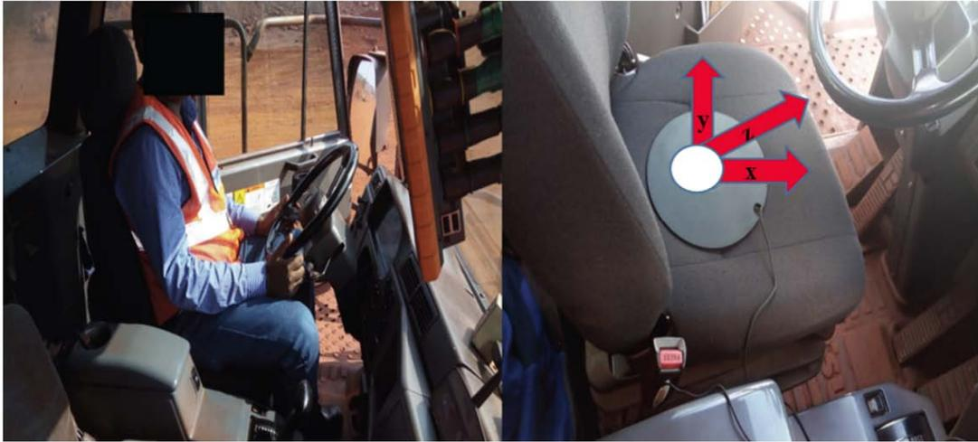
**Figure 2:** A dumper operator's seat cabin and seat pad accelerometer with the measurement axes.
