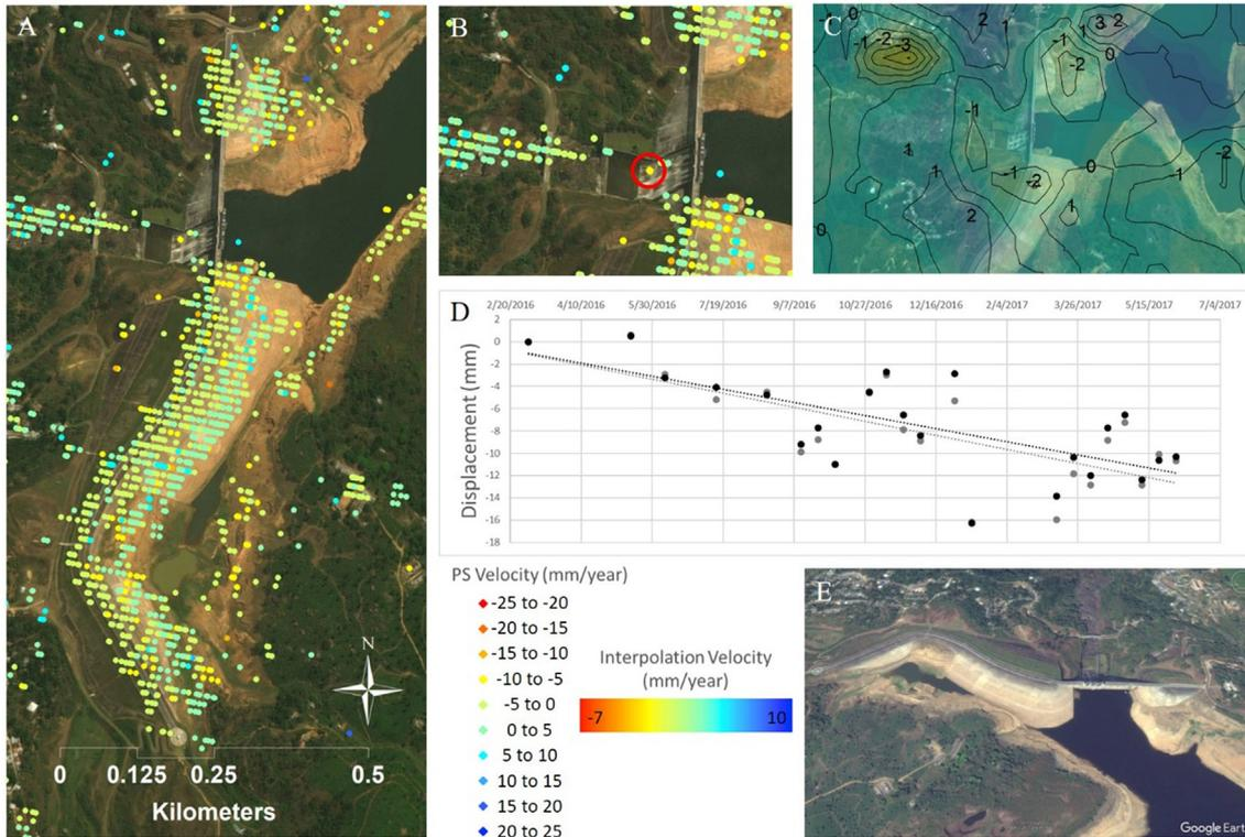
**Fig. 6.** Upper Sholayar Dam. (A) Results from PSI technique. PS are individual points measuring velocity (mm/y) ranging from -25 mm/y (red) to 25 mm/y (blue). (B) Close-up of PS points on Upper Sholayar Dam. (C) Kriging interpolation of PSI results (contour interval = 1 mm/y). Interpolation velocity ranges from -7 mm/y (red) to 10 mm/y (blue). (D) Displacement-time series of two PS points in red circle from (B). (E) Google Earth view of Upper Sholayar Dam.
