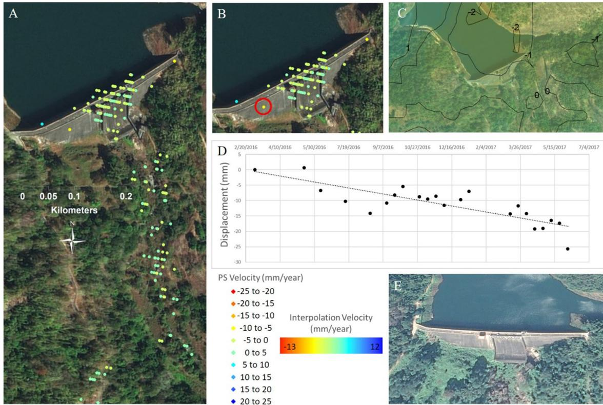
**Fig. 4.** Idamalayar Dam. (A) Results from PSI technique. PS are individual points measuring velocity (mm/year) ranging from -25 mm/year (red) to 25 mm/year (blue). (B) Close-up of PS points on Idamalayar Dam. (C) Kriging interpolation of PSI results (contour interval = 1 mm/year). Interpolation velocity ranges from -13 mm/year (red) to 12 mm/year (blue). (D) Displacement-time series of PS point in red circle from Fig. 4(B). (E) Google Earth view of the Idamalayar Dam.
