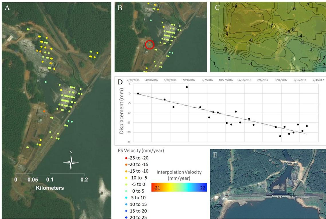
**Fig. 5.** Malankara Dam. (A) Results from PSI technique. PS are individual points measuring velocity (mm/year) ranging from -25 mm/year (red) to 25 mm/year (blue). (B) Close-up of PS points on Malankara Dam. (C) Kriging interpolation of PSI results (contour interval = 1 mm/year). Interpolation velocity ranges from -21 mm/year (red) to 22 mm/year (blue). (D) Displacement-time series of PS point in red circle from (B). (E) Google Earth view of the Malankara Dam.
