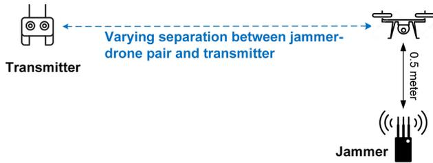
FIGURE 1. Experimental setup to obtain effective jamming range.
