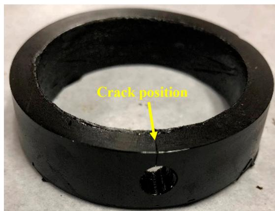
(c) Sample with crack after the test
