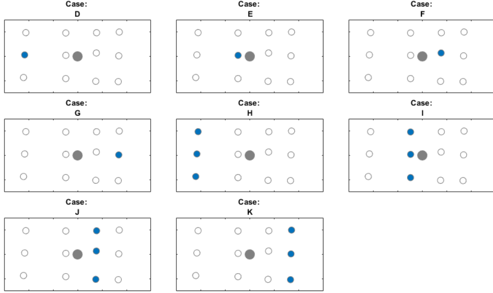
Figure 4.6: Illustration of the wave gauges used for the cases described in Table 4.3 where waves propagate from left-to-right.
