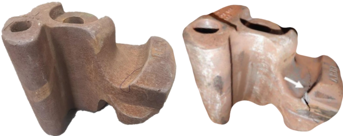
Figure 3: Intact knuckle (left) and knuckle exhibiting fatigue crack in the pulling lug (right) [2]
