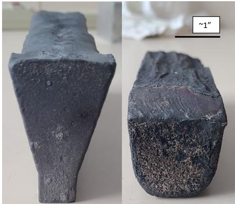
Figure 15: Michigan Tech cast Grade-E y-block (left) and a cast Grade-E keel block provided by Amsted Rail (right). The keel blocks were machined into rotary bend fatigue samples to provide baseline data.
