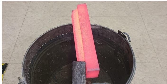
Figure 16: A WAM printed sample just after austenitization and before being quenched.
