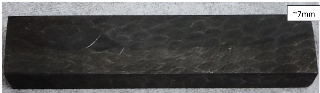
Figure 35: Highly visible weld bead profiles on a WAM build after an hour-long submersion in a dilute HCl solution.
