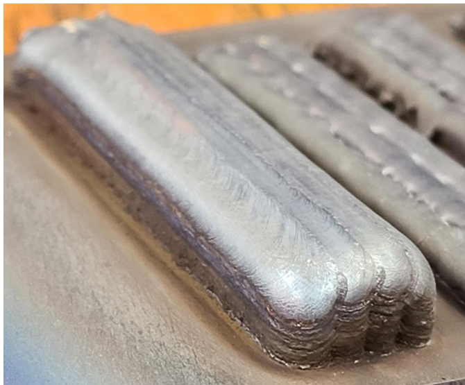
Figure 13: A "half" 40 mm long sample with a shorter print time for property testing. The substrate is a 1018 mild steel plate.
