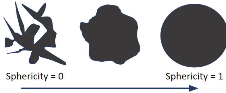
Figure 33: Exaggerated representation of sphericity. Jagged edges on less spherical pores are more likely to initiate cracks.
