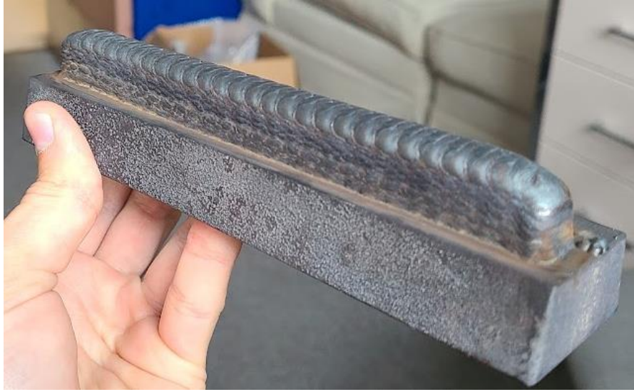
Figure 14: WAMA 160 mm long WAM print, which can be machined into two hour-glass rotary bend fatigue samples. Substrate is a Grade-E y-block riser.
