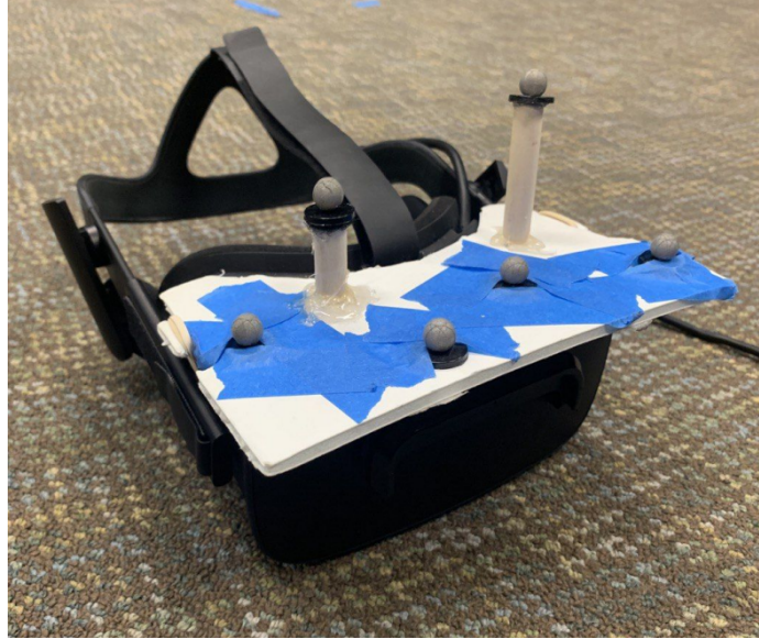
Figure 3.3: Oculus CV1 with Vicon tracker markers
