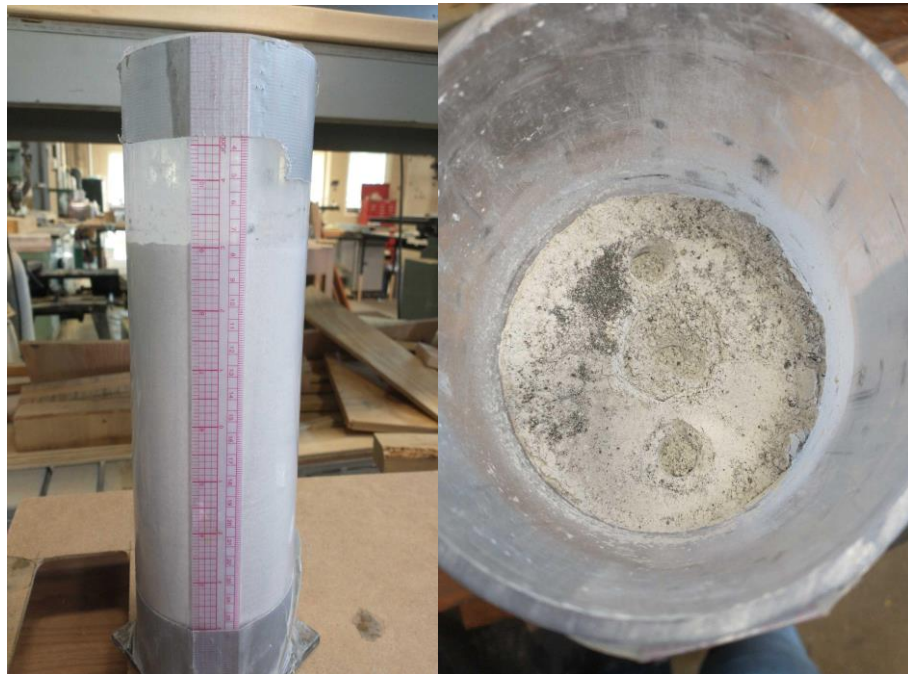
Figure 4-4 Compacted regolith cylinder (1.76 g/cc or 82.1%)
