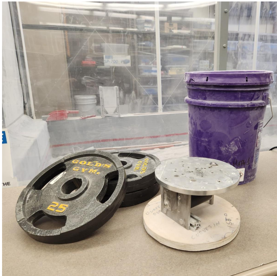
Figure 3-2 Surface pressure testing equipment
