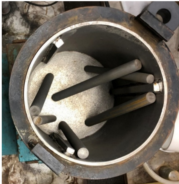
Figure 2.3 Picture of Carrier and Rods of a Rod Mill
