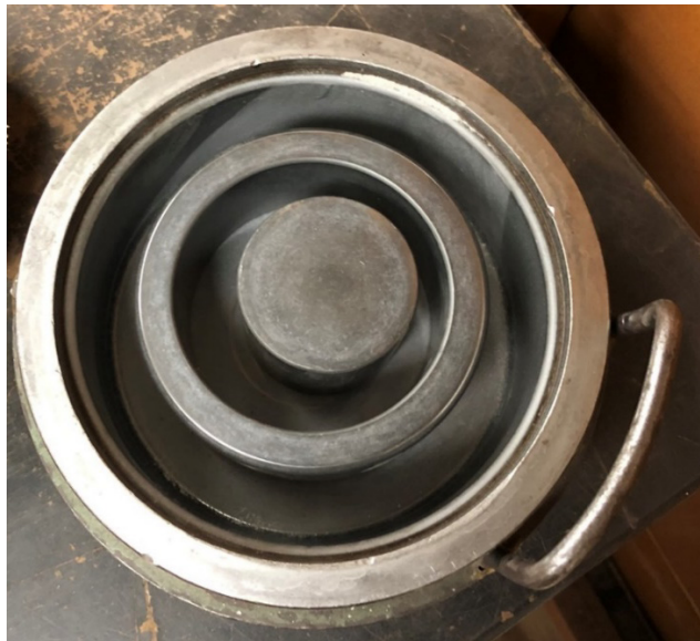
Figure 2.4 Inside the Carrier of a Puck Mill
