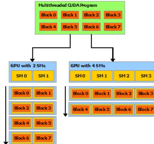
**Figure 2.7:** GPU Multithreading [26]
