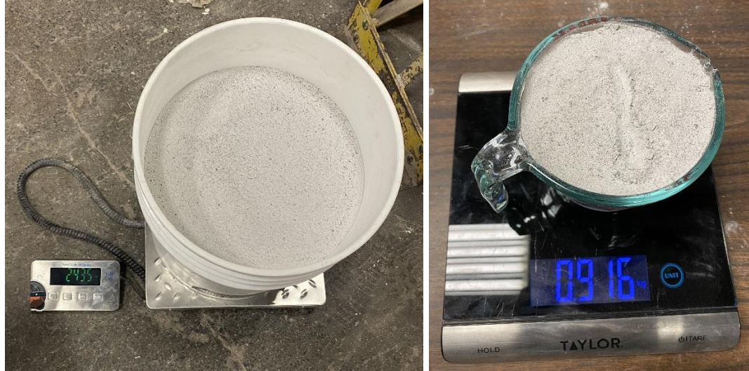
Figures 10 & 11: (1) Weighing the dry sample of regolith to determine wt.% of water. (2) Post-mixture weighing small desiccated mixed samples for water content validation.
