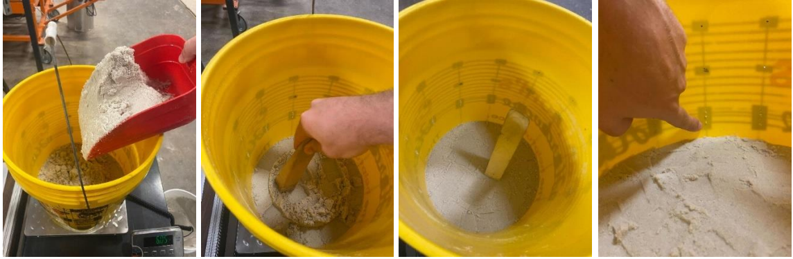
Figures 12 - 15: Test setup steps number 1, adding mixed silica sand sample, uniformly compacting 2-to-3-inch layers until the first thermocouple layer is reached.
