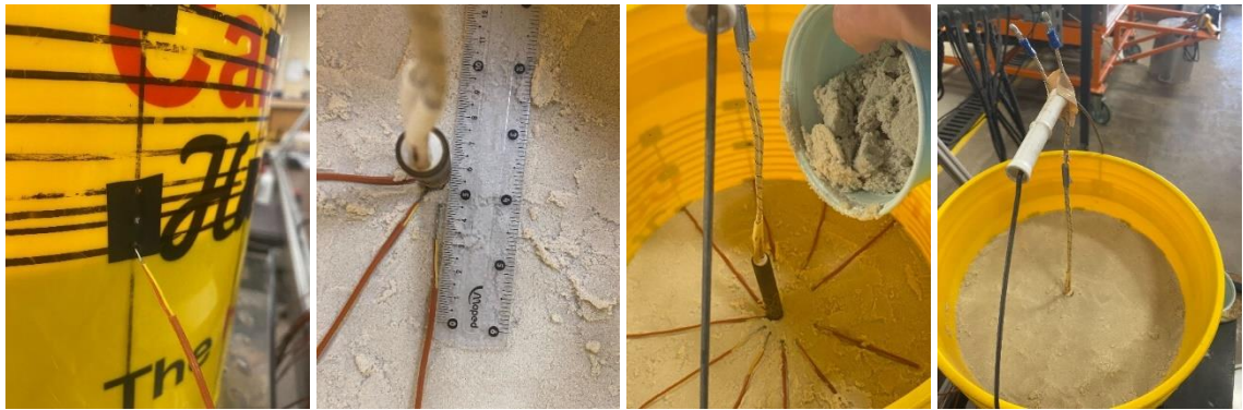
Figures 16 - 19: Test setup steps 2 through 9, inserting thermocouples and measuring their placement in mm relative to the cartridge heater placement, adding mixed silica sand sample and compacting layers to the top of the cartridge heater.
