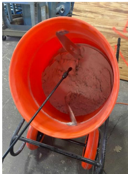
Figure 9: Procedure for mixing a sample with an even distribution of a specific weight percentage of water.
