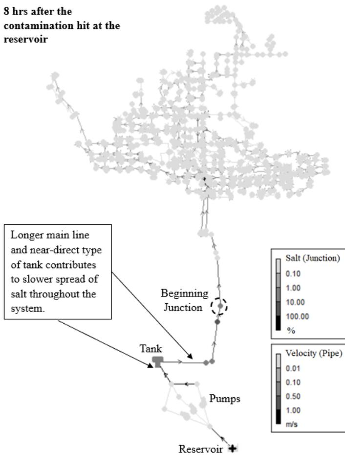
Figure 2-20. Salt intrusion contour of System 9 at Beginning Junction Contamination Hour for S-1 of the gradual salt intrusion event.
