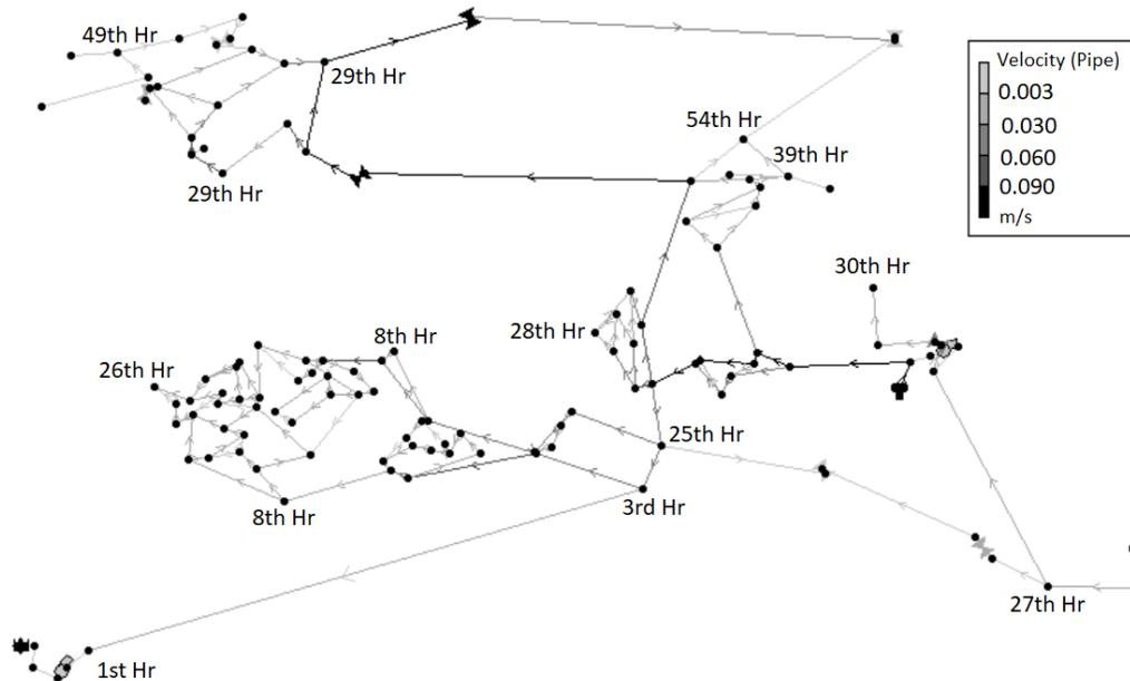
Figure 2-7. Hour of salt intrusion contour of System 6 for the instantaneous salt intrusion event.
