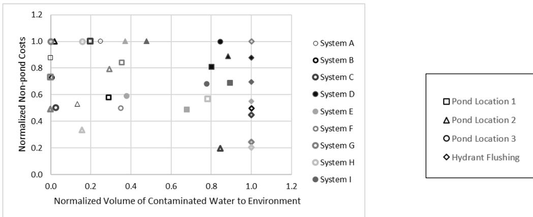
Figure 3-4. Normalized non-pond costs vs. normalized volume of contaminated water to environment for different pond locations.
