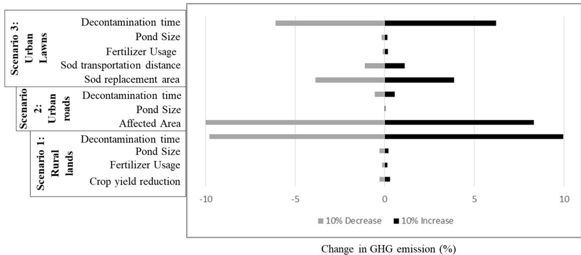
Figure 4-4. Sensitivity analysis for key inputs to containment pond and hydrant flushing at various scenarios.
