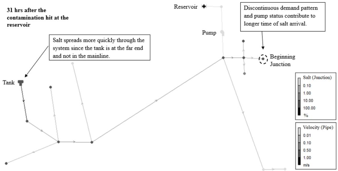
Figure 2-15. Salt intrusion contour of System 3 at Beginning Junction Contamination Hour for S-1 of the gradual salt intrusion event.
