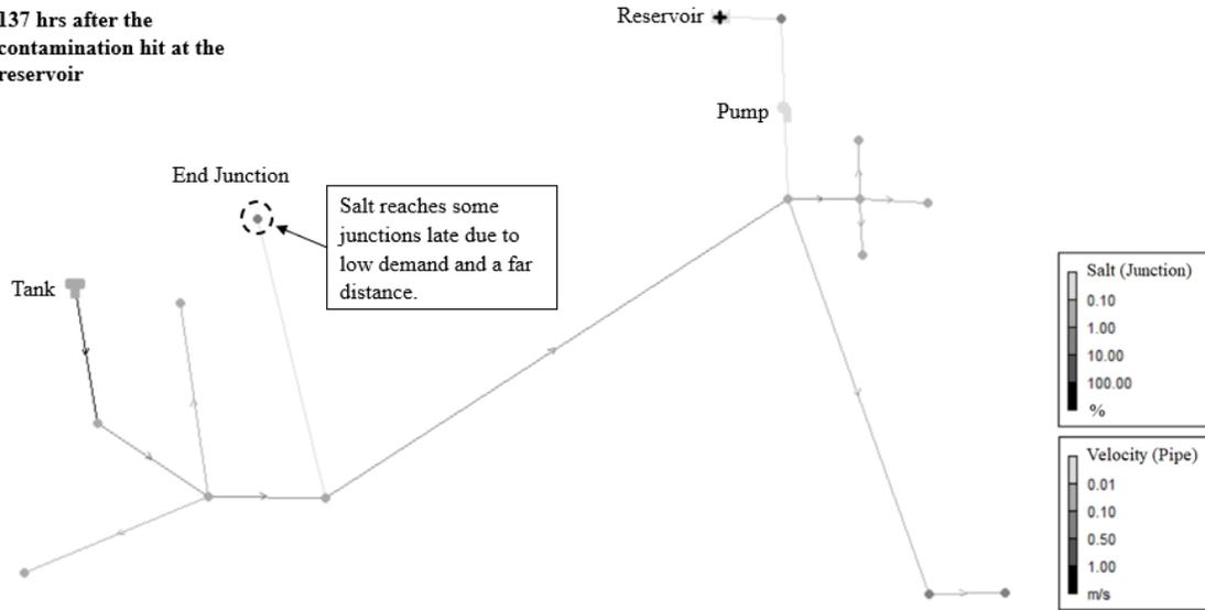
Figure 2-17. Salt intrusion contour of System 3 at End Junction Contamination Hour for S-12 of the gradual salt intrusion event.
