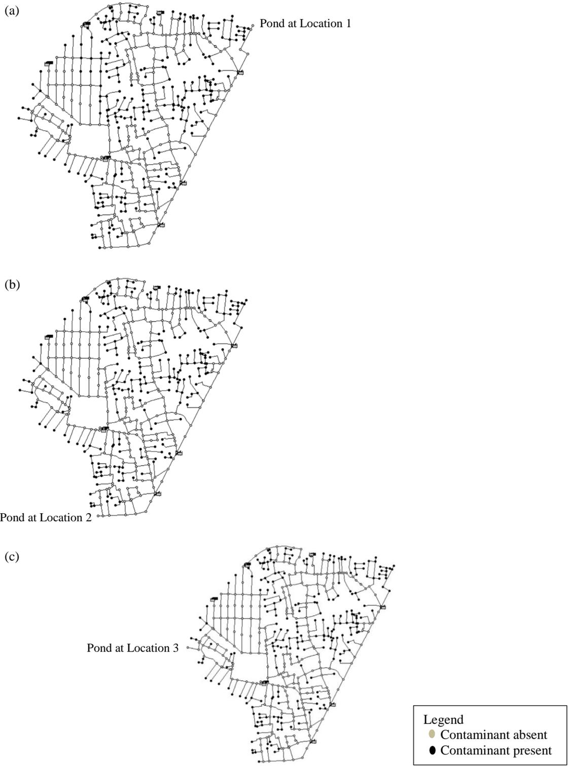
Figure A.8. System H at pond maximum capacity for the pond at (a) Pond Location 1, (b) Pond Location 2 and (c) Pond Location 3.
