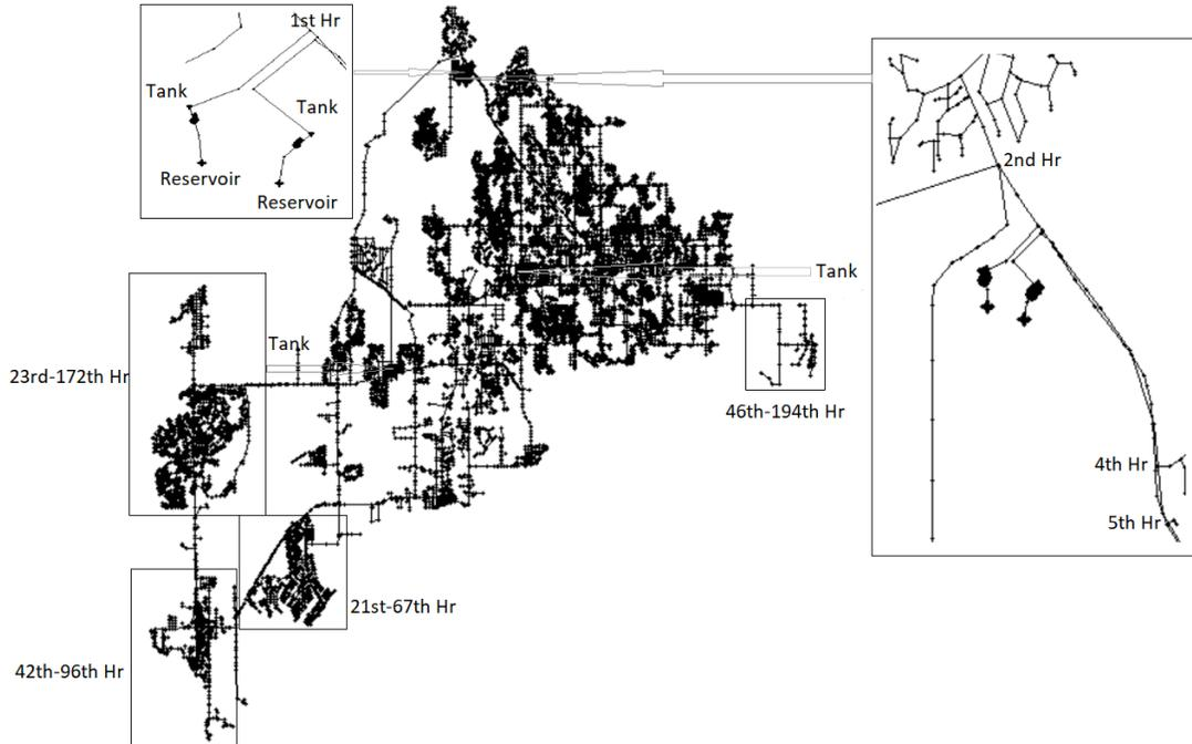
Figure 2-11. Hour of salt intrusion contour of System 10 for the instantaneous salt intrusion event.
