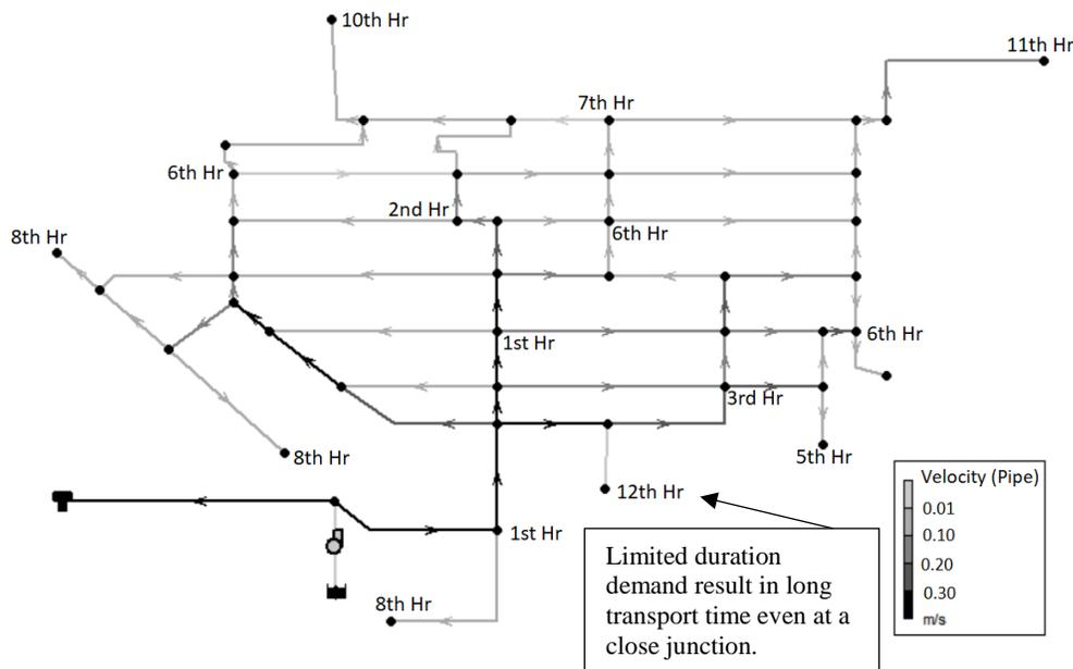
Figure 2-6. Hour of salt intrusion contour of System 5 for the instantaneous salt intrusion event.
