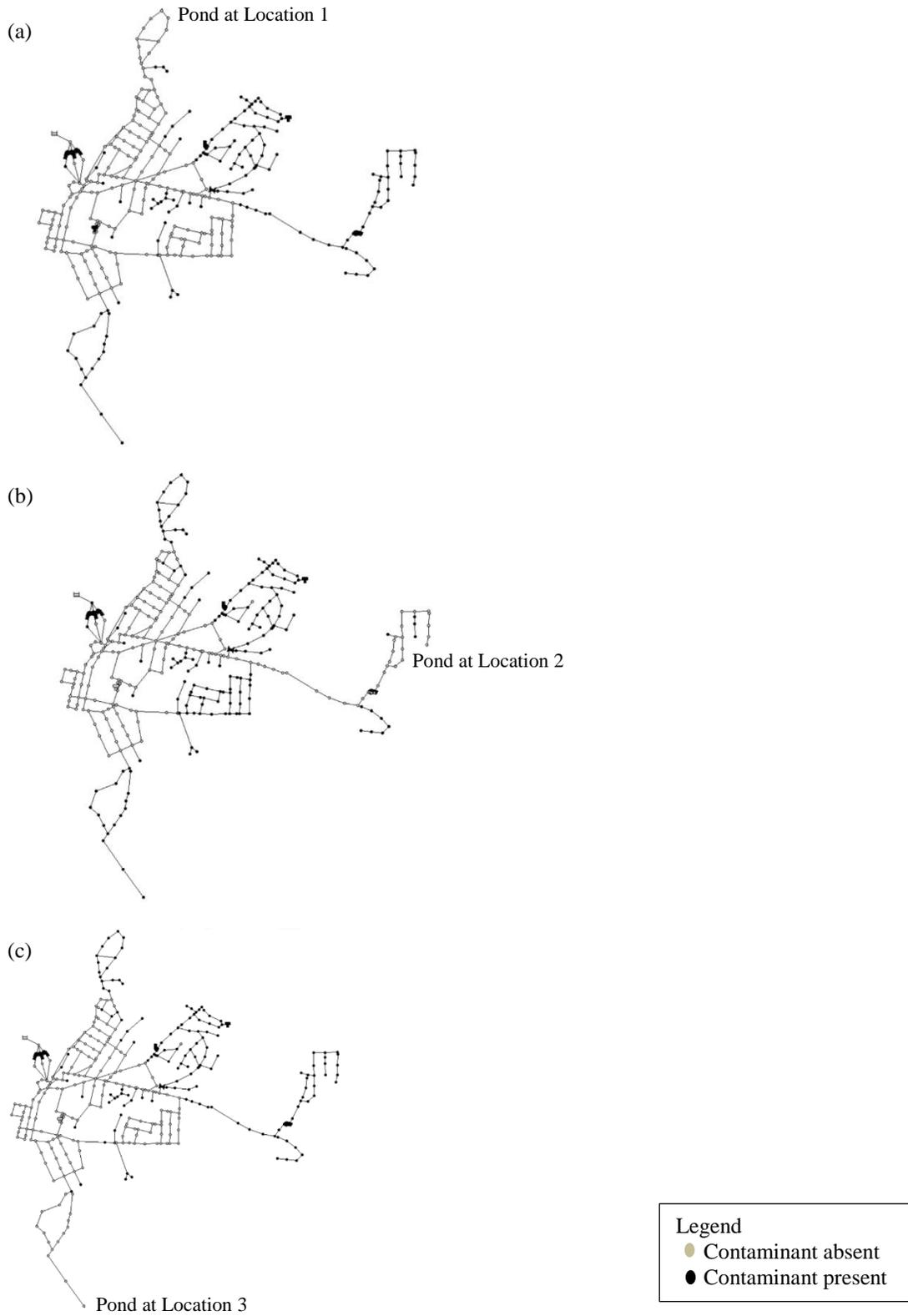
Figure A.5. System E at pond maximum capacity for the pond at (a) Pond Location 1, (b) Pond Location 2 and (c) Pond Location 3.
