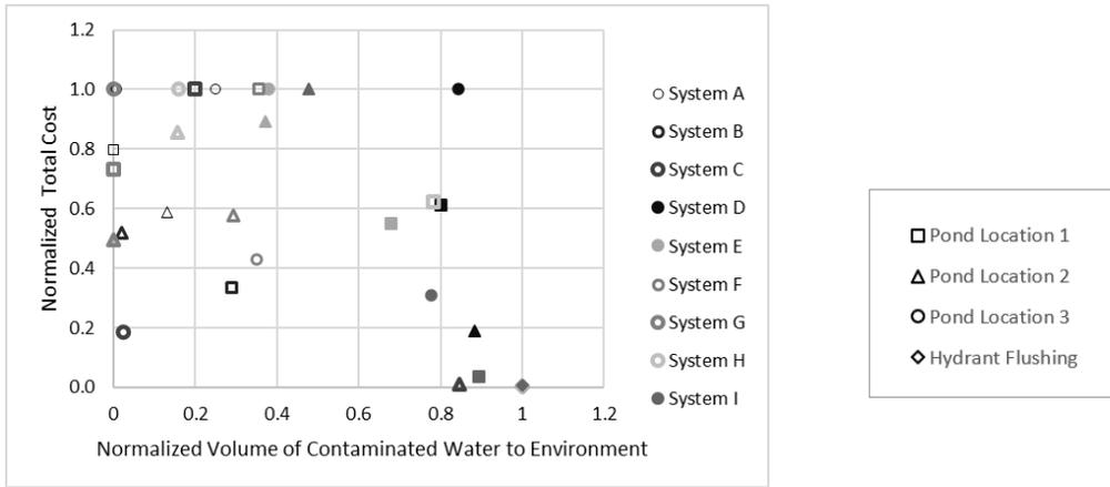
Figure 3-3. Normalized pond total cost vs. normalized volume of contaminated water to the environment for different pond locations.
