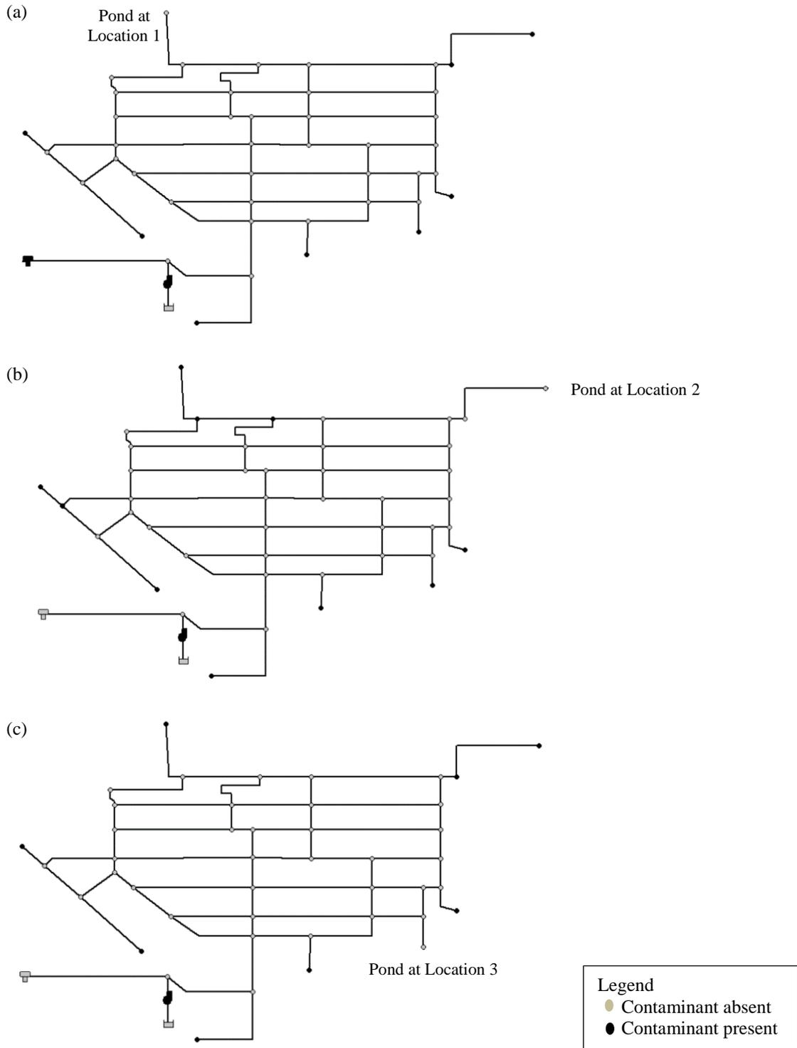
Figure A.2. System B at pond maximum capacity for the pond at (a) Pond Location 1, (b) Pond Location 2 and (c) Pond Location 3.
