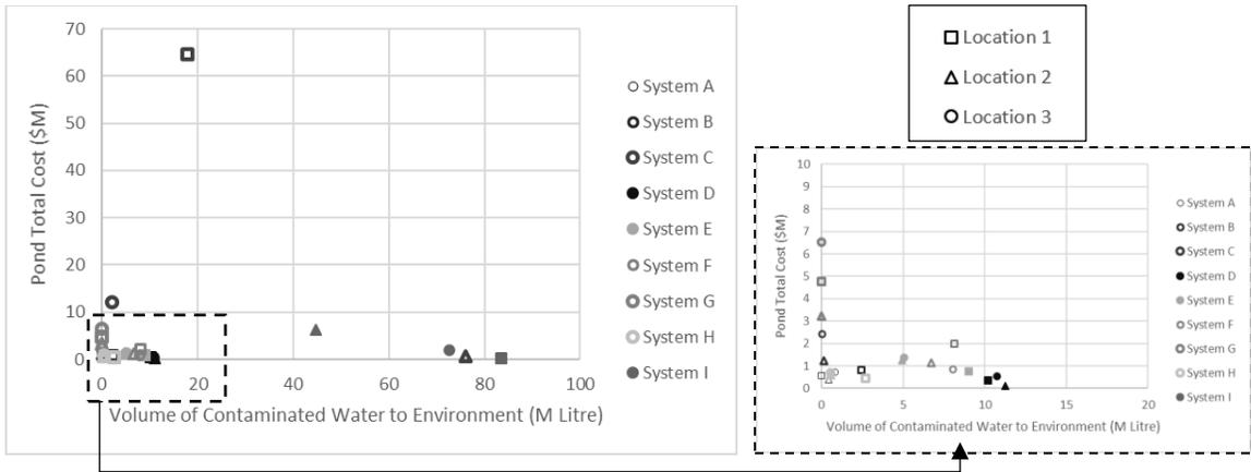
Figure 3-2. Pond total cost vs. volume of contaminated water to the environment for different pond locations.
