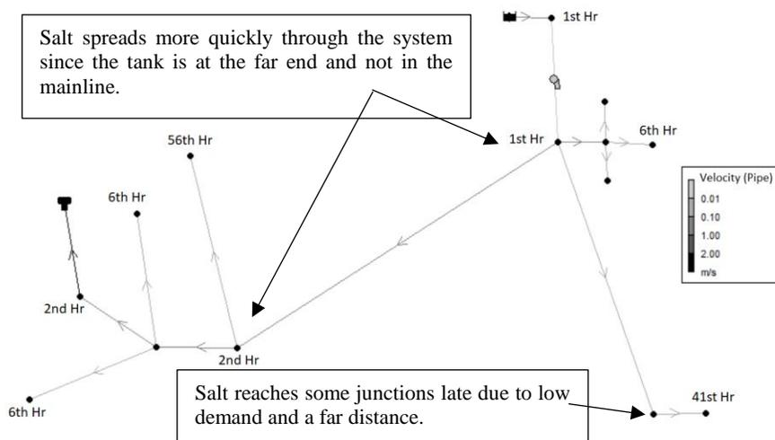
Figure 2-4. Hour of salt intrusion contour of System 3 for the instantaneous salt intrusion event.
