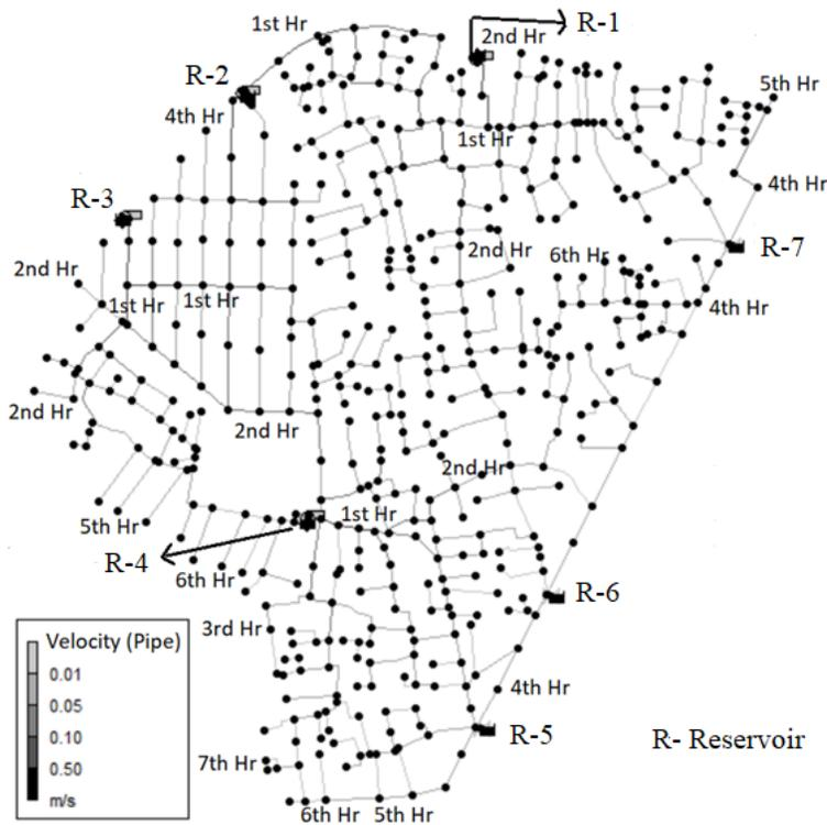
Figure 2-14. Hour of salt intrusion contour of System 13 for the instantaneous salt intrusion event.
