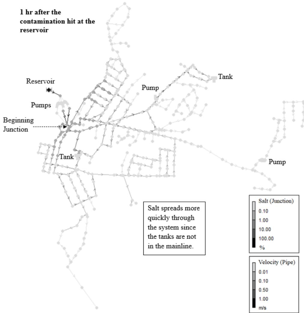
Figure 2-18. Salt intrusion contour of System 8 at Beginning Junction Contamination Hour for S-7 of the gradual salt intrusion event.
