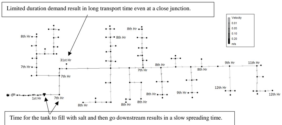
Figure 2-2. Hour of salt intrusion contour of System 1 for instantaneous salt intrusion event.
