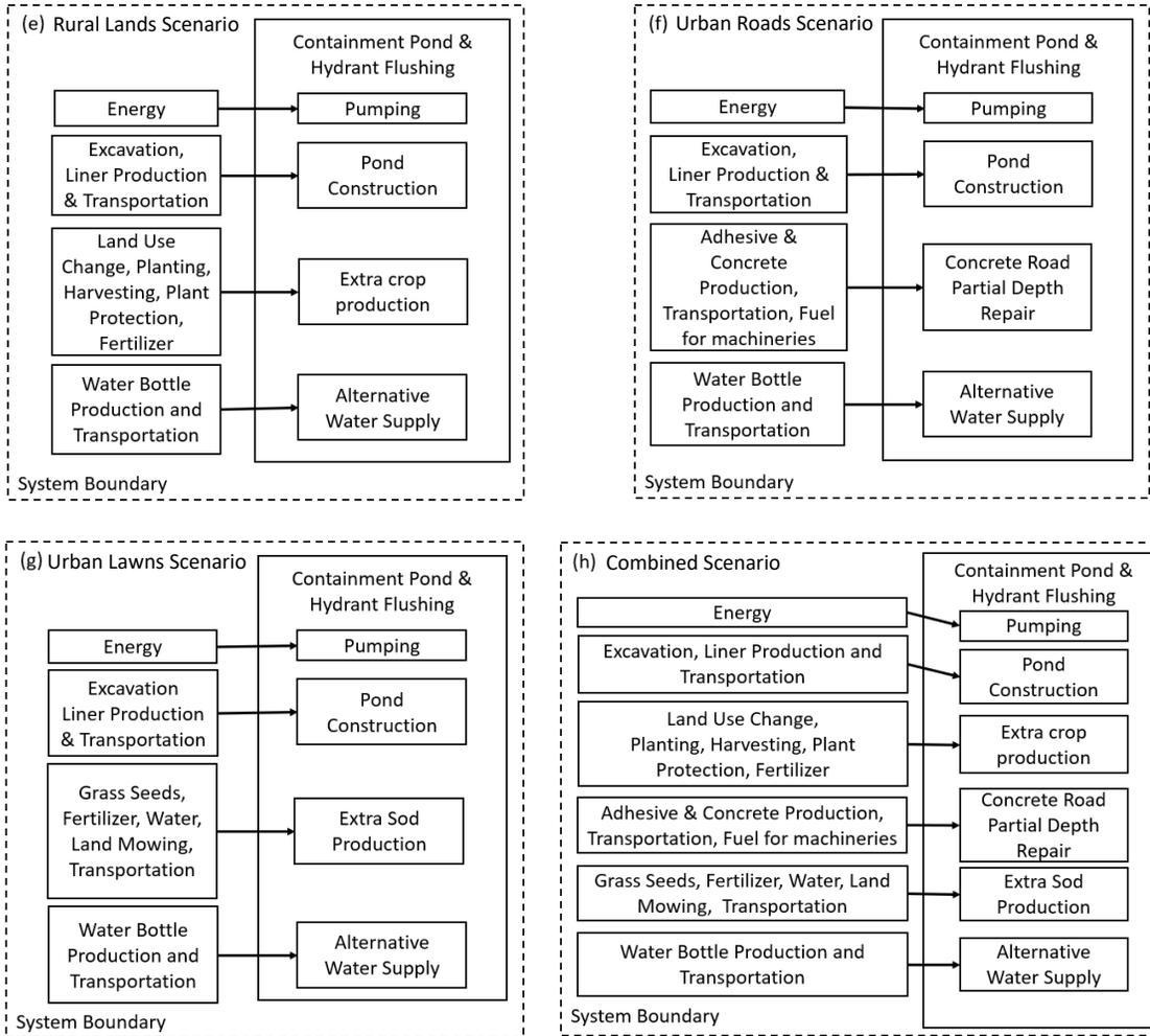
Figure 4-2 (continued). System boundaries used in the LCA of the WDS decontamination using hydrants (a, b, c, d) and a containment pond and hydrants (e, f, g, h) under various scenarios.
