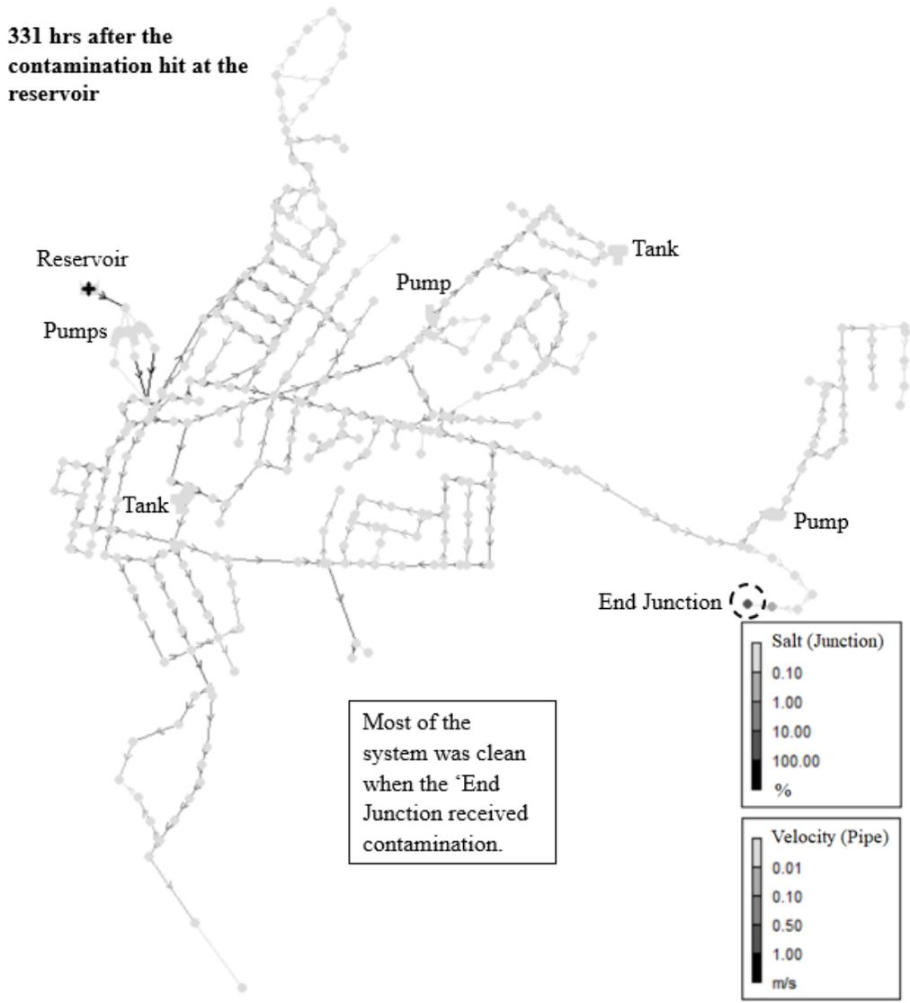
Figure 2-19. Salt intrusion contour of System 8 at End Junction Contamination Hour for S-1 of the gradual salt intrusion event.
