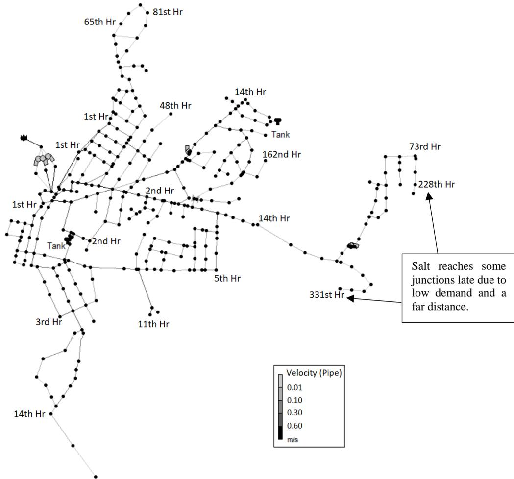
Figure 2-9. Hour of salt intrusion contour of System 8 for the instantaneous salt intrusion event.
