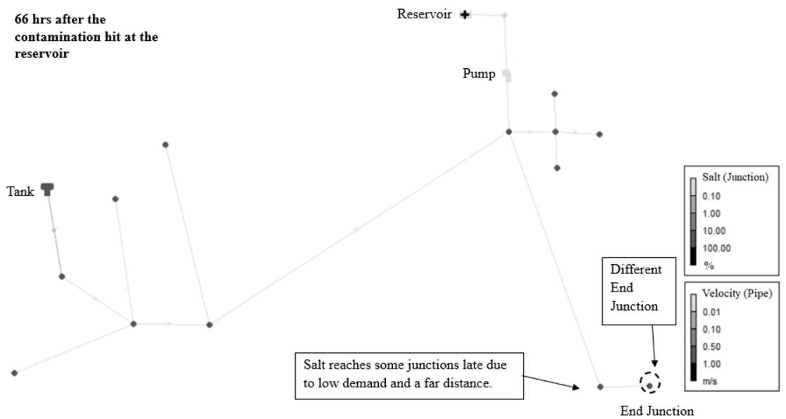
Figure 2-16 Salt intrusion contour of System 3 at End Junction Contamination Hour for S-1 of the gradual salt intrusion event.
