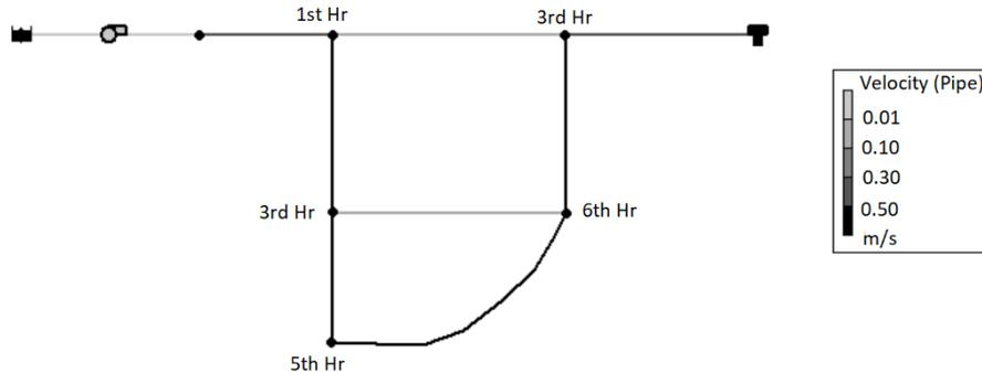
Figure 2-5. Hour of salt intrusion contour of System 4 for the instantaneous salt intrusion event.
