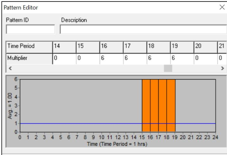
Figure 1-2. An example of industrial water demand pattern in pattern editor of EPANET.
