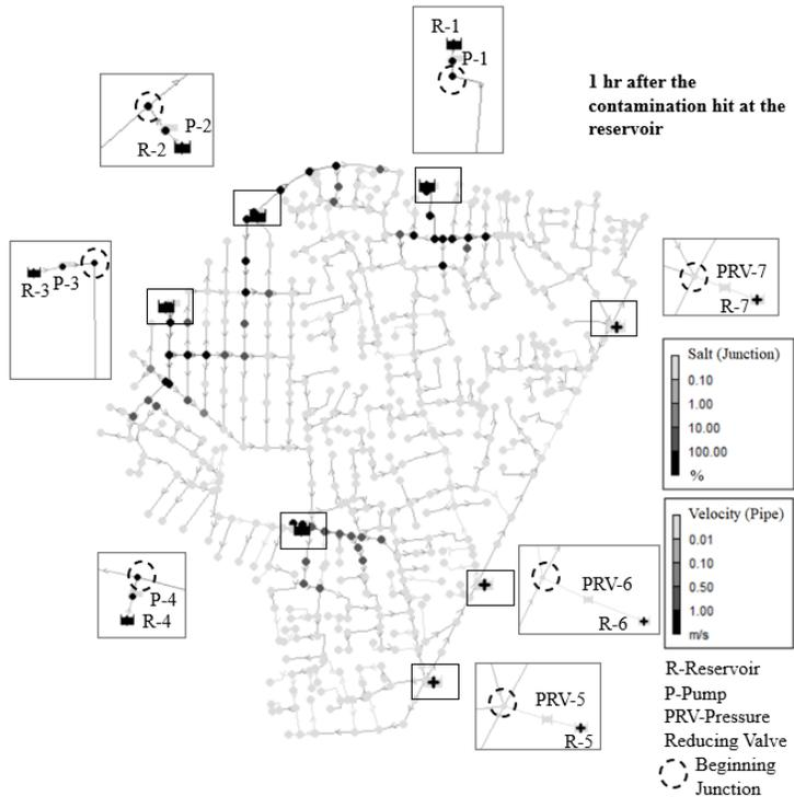
Figure 2-22. Salt intrusion contour of System 13 at Beginning Junction Contamination Hour for S-1 of the gradual salt intrusion event.
