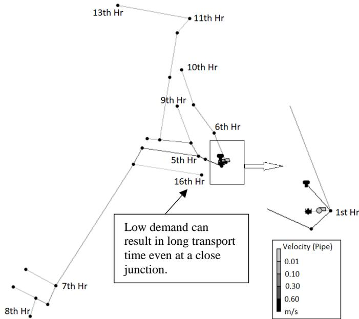
Figure 2-3. Hour of salt intrusion contour of System 2 for the instantaneous salt intrusion event.
