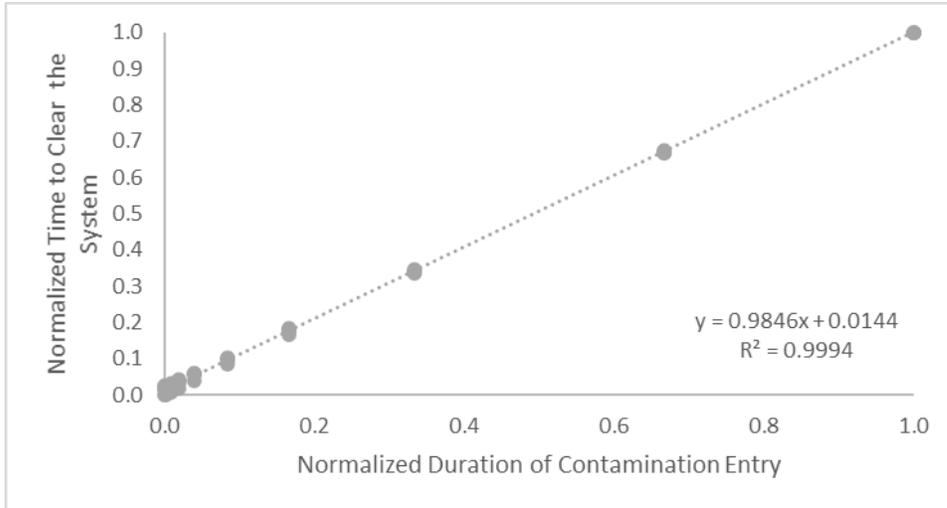
Figure 2-25. The trend line for time to clear any system in terms of salt contamination duration.
