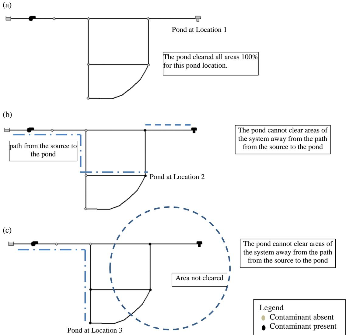
Figure A.1. System A at pond maximum capacity for the pond at (a) Pond Location 1, (b) Pond Location 2, and (c) Pond Location 3. The same thing holds for the other systems as seen in Table 3-3.
