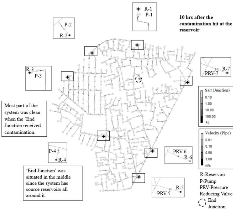
Figure 2-23. Salt intrusion contour of System 13 at End Junction Contamination Hour for S-1 of the gradual salt intrusion event.
