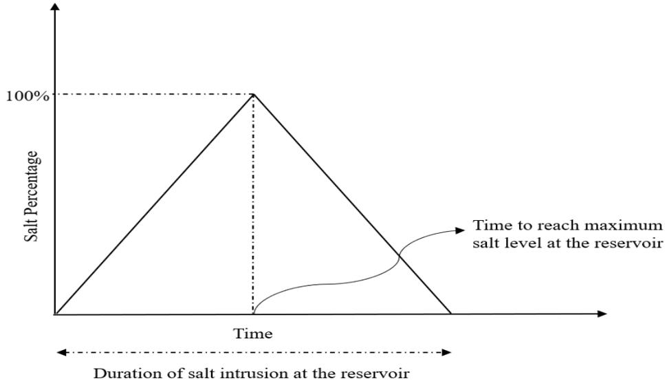
Figure 2-1. Salt percentage input over time following the same rate of change for the gradual salt intrusion event.
