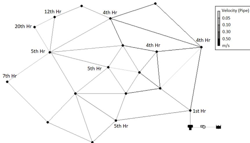
Figure 2-12. Hour of salt intrusion contour of System 11 for the instantaneous salt intrusion event.
