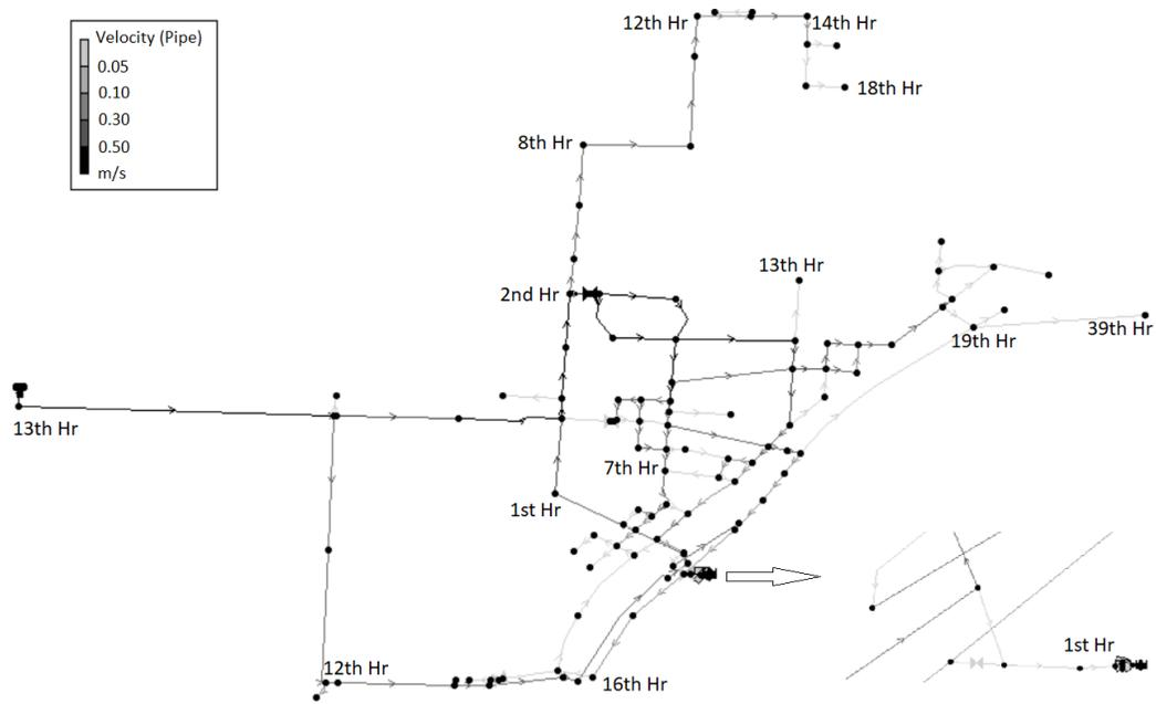
Figure 2-8. Hour of salt intrusion contour of System 7 for the instantaneous salt intrusion event.
