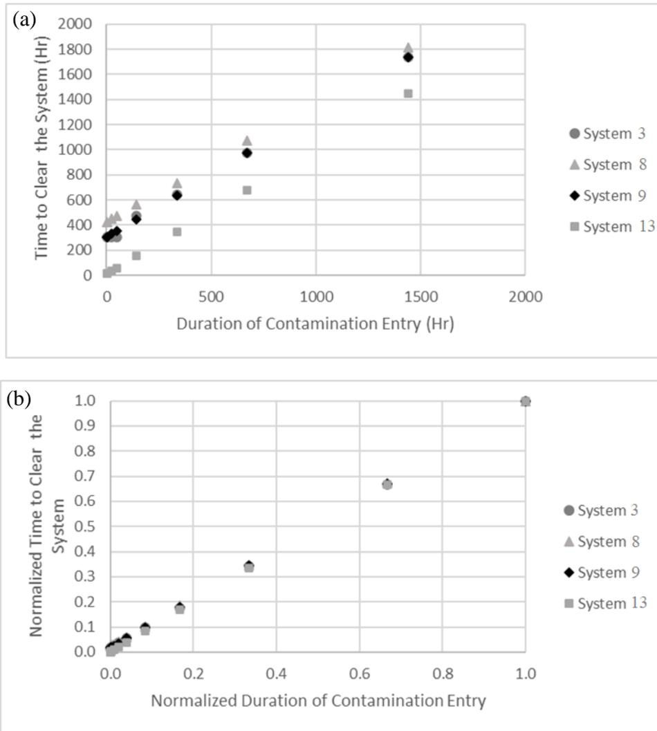
Figure 2-24. Systems comparison in terms of salt contamination termination (a) in actual scale, (b) in normalized scale.
