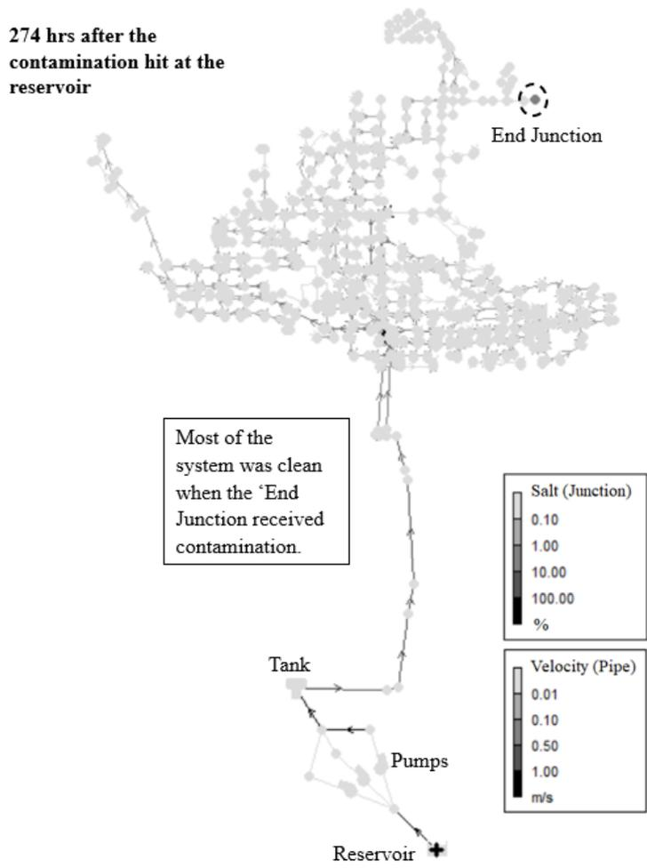
Figure 2-21. Salt intrusion contour of System 9 at End Junction Contamination Hour for S-1 of the gradual salt intrusion event.
