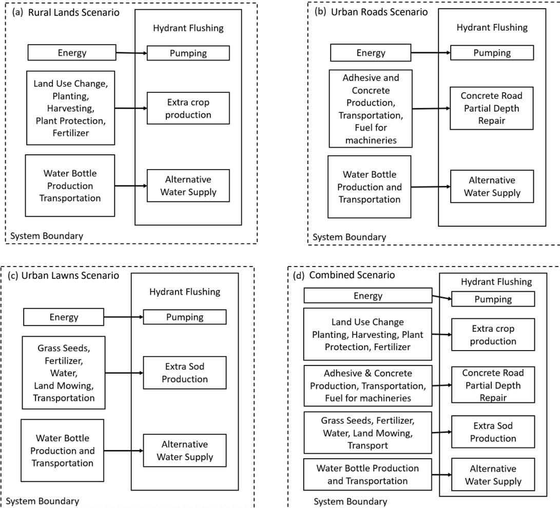
Figure 4-2. System boundaries used in the LCA of the WDS decontamination using hydrants (a, b, c, d) and a containment pond and hydrants (e, f, g, h) under various scenarios.
