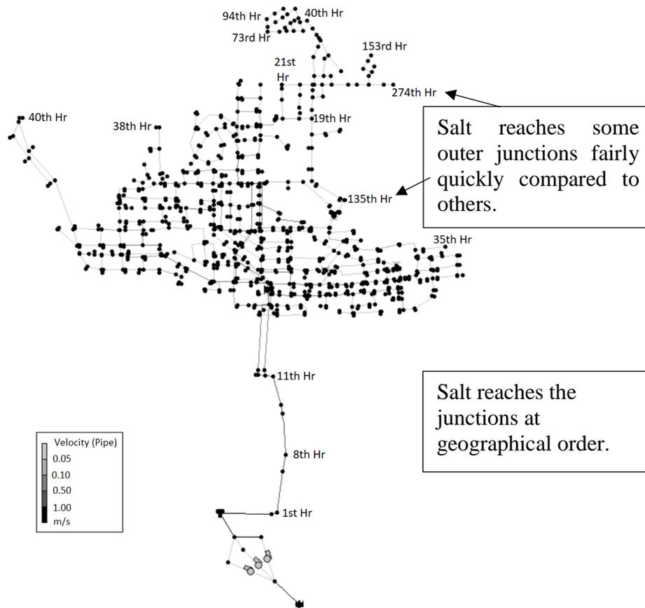
Figure 2-10. Hour of salt intrusion contour of System 9 for the instantaneous salt intrusion event.
