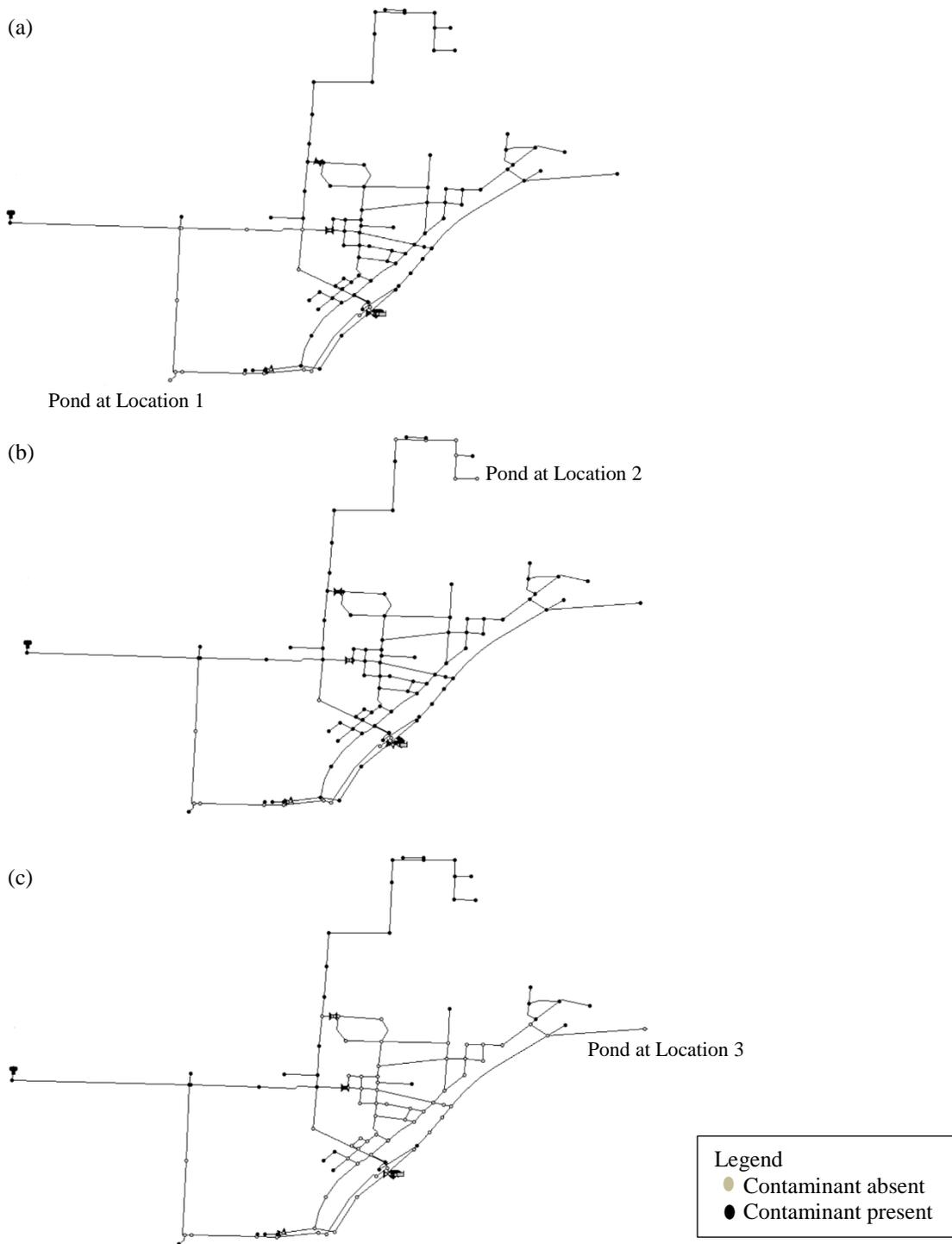
Figure A.4. System D at pond maximum capacity for the pond at (a) Pond Location 1, (b) Pond Location 2 and (c) Pond Location 3.
