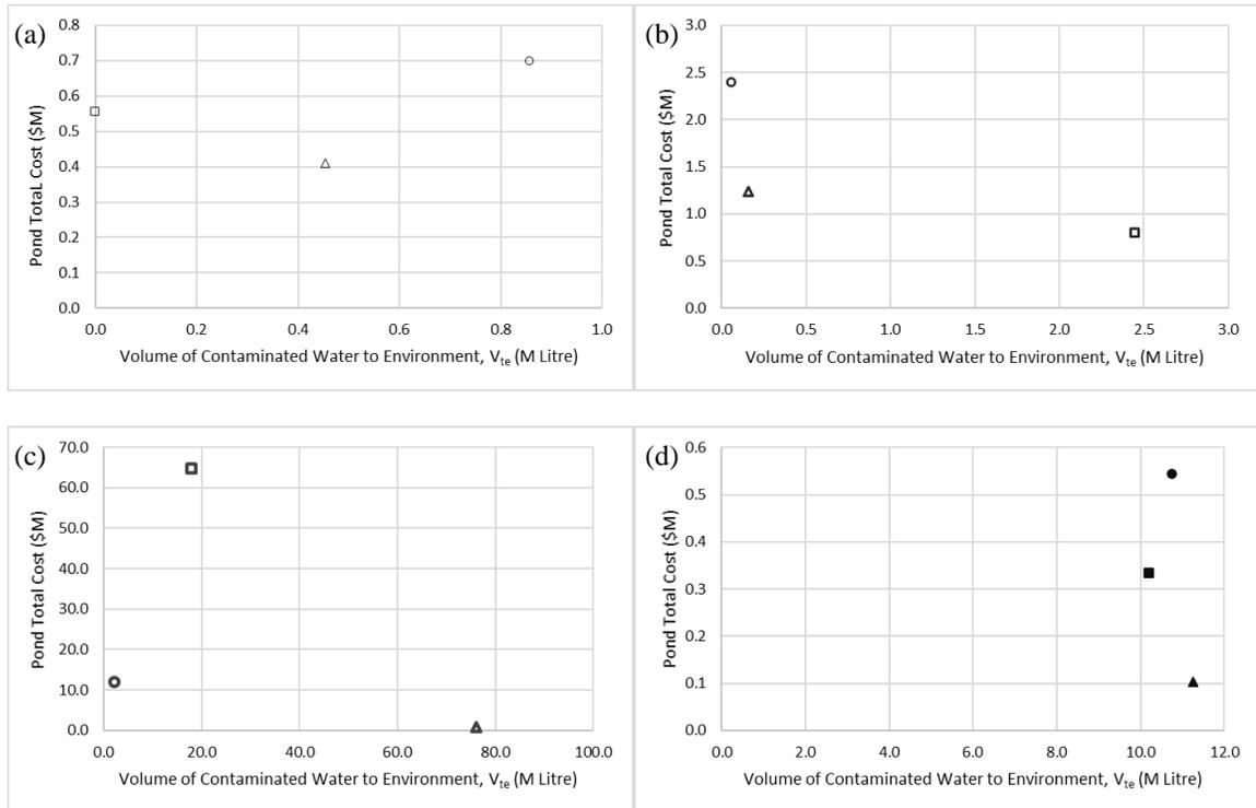
Figure 3-1. Pond total cost vs. volume of contaminated water to environment corresponding to (a) System A, (b) System B, (c) System C, (d) System D, (e) System E, (f) System F, (g) System G, (h) System H, and (i) System I.
