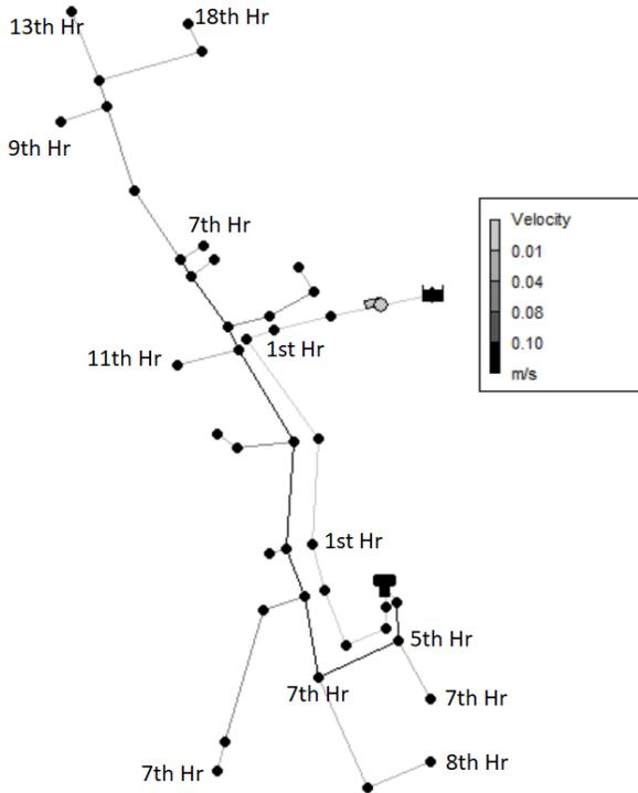
Figure 2-13. Hour of salt intrusion contour of System 12 for the instantaneous salt intrusion event.
