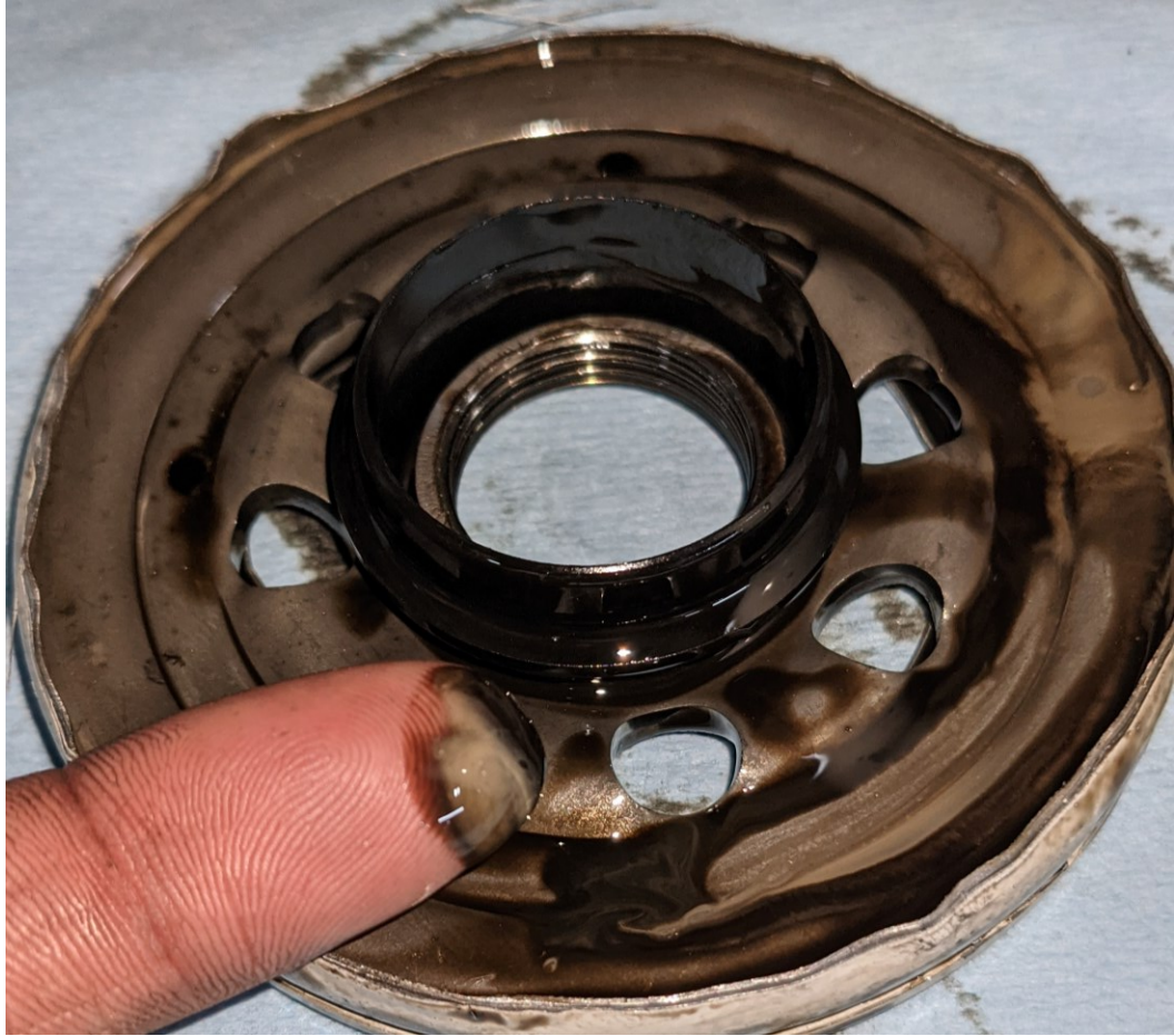
Figure 59. Closeup of Creamy Oil in Oil Filter
