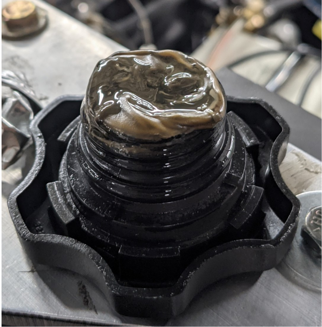
Figure 58. Oil Fill Cap with Creamy Oil
