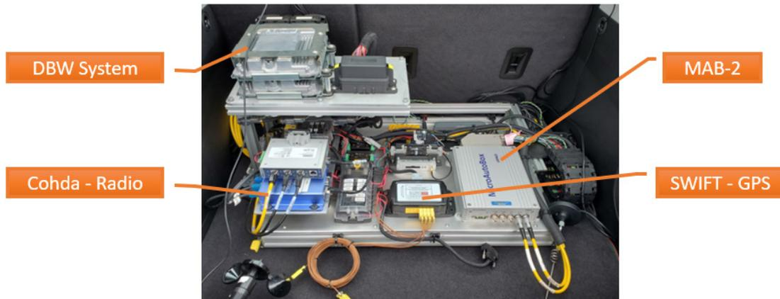
Figure 5 Vehicle Instrumentation in boot
