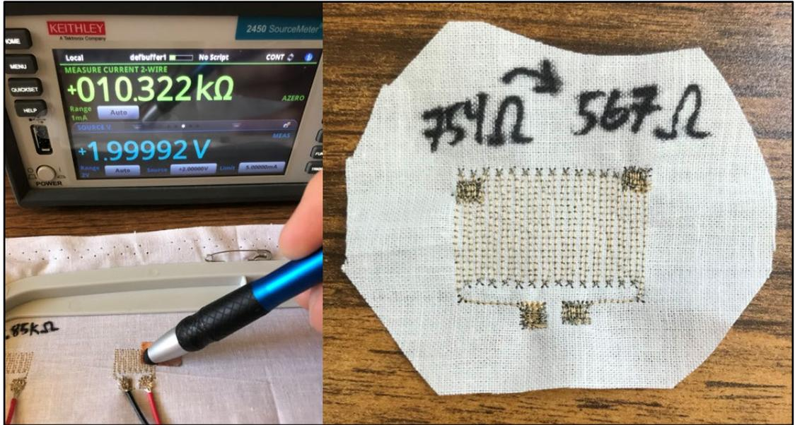
**Figure 4.9:** Experimental setup. (a) Measuring where to create a short circuit (left) and (b) a resistor after having short circuits created (right).
