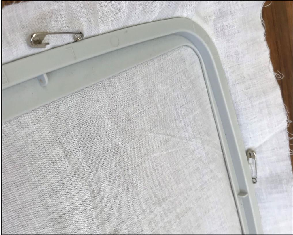
**Figure 4.8:** Use of safety pins to prevent fabric movement within embroidery hoop.
