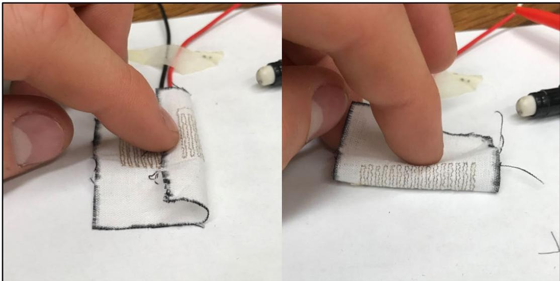
**Figure 5.6 a & b:** Folding the resistor parallel to (left) and perpendicular to (right) the embroidered conductive flow path tines.
