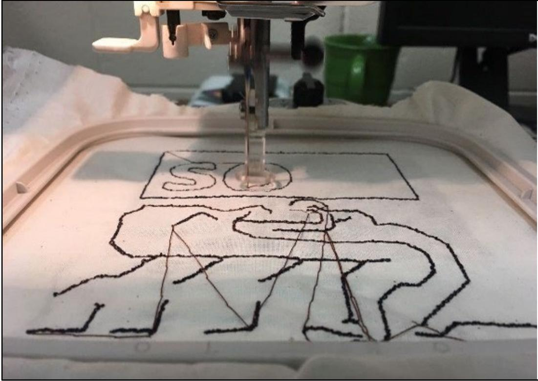
**Figure 1.2:** Embroidery machine in operation [12]. This manufacturing process can be used to create electronic circuits and aesthetic designs.
