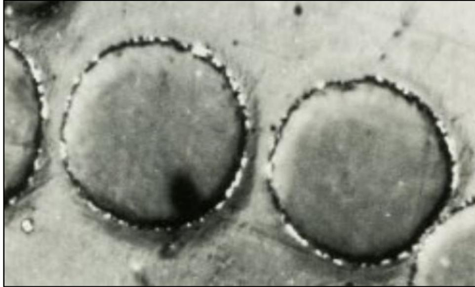
**Figure 4.3:** Cross section of the silver coating over nylon base for 44/12 + 113/32 PET thread [43]
