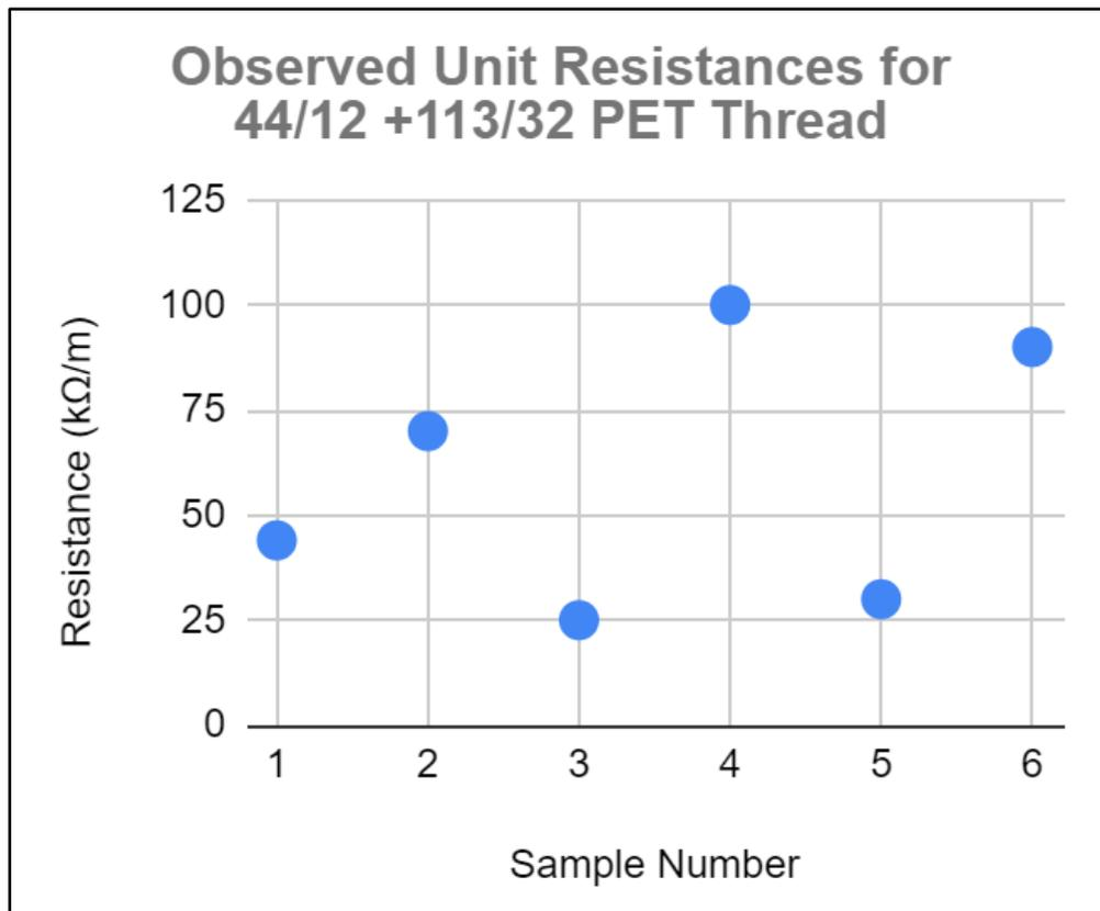
**Figure 4.4:** Inconsistencies in the unit resistance between batches of the silver-coated nylon thread 44/12 + 113/32 PET.
