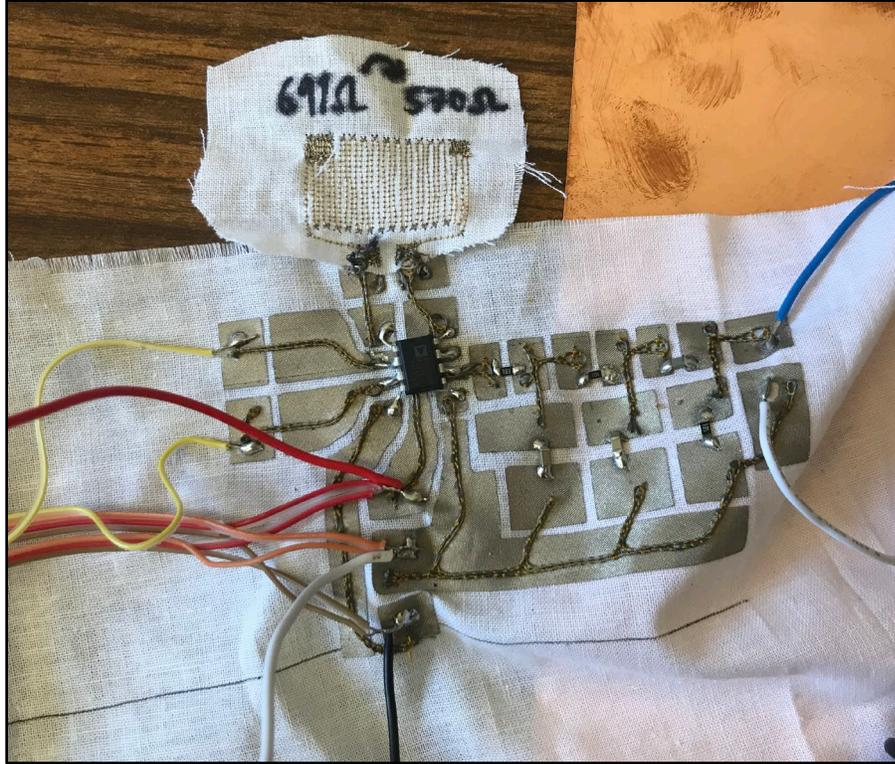
**Figure 6.4:** Touch sensing device with a flexible resistor attached.
