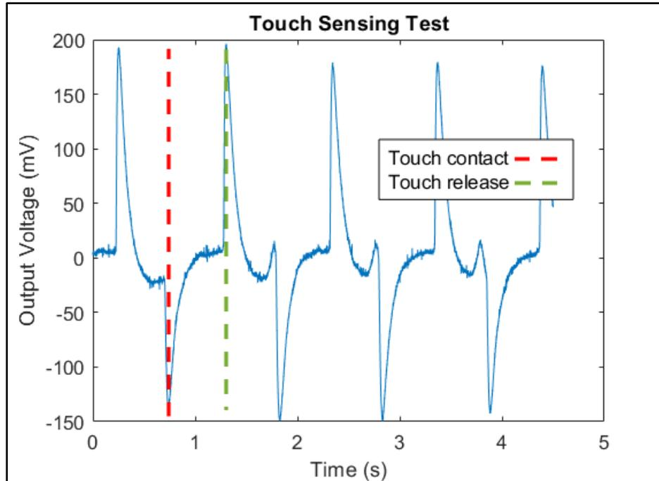
**Figure 6.6:** Touch sensing test results.
