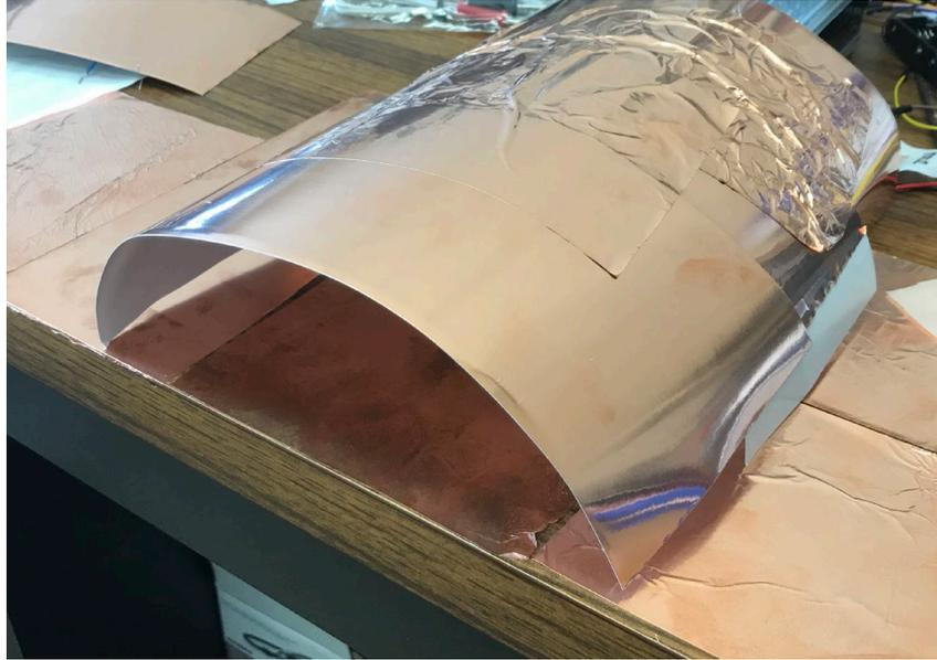
**Figure 6.5:** Copper tent to provide shielding for the prototype device.
