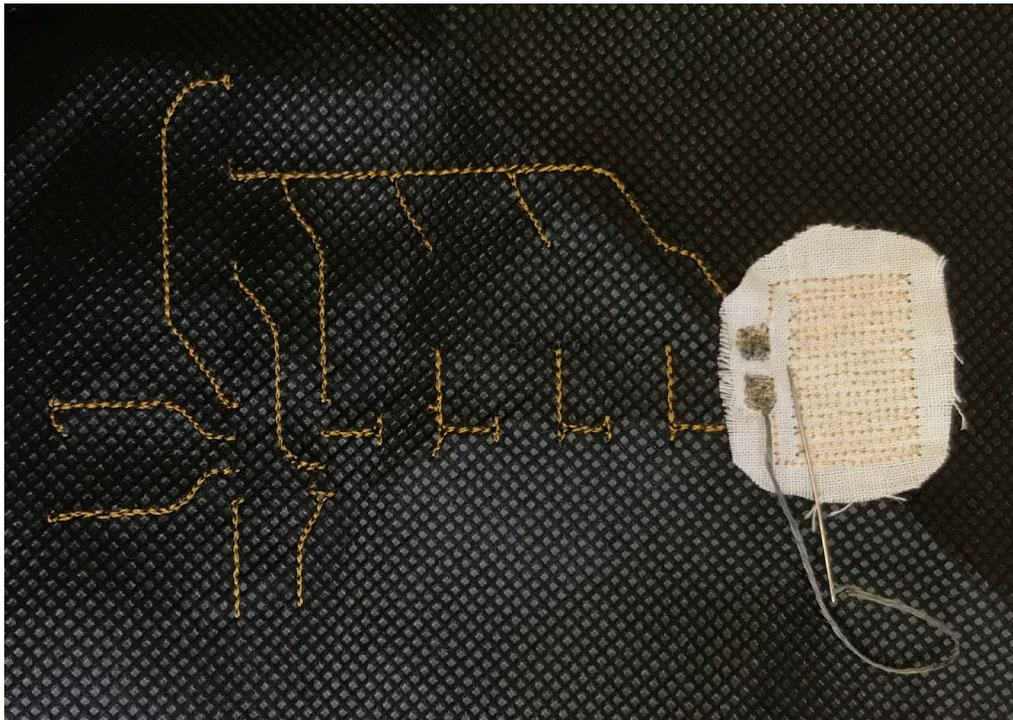
**Figure 4.6:** A resistor attached to an embroidered circuit via hand sewing.
