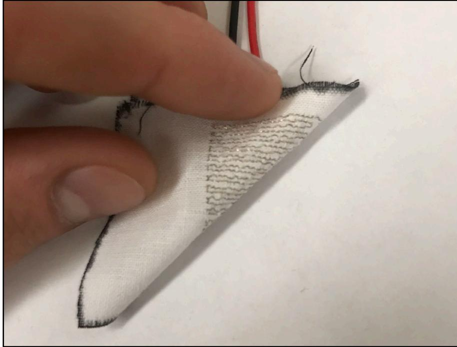
**Figure 5.4:** Diagonal fold method used for testing.
