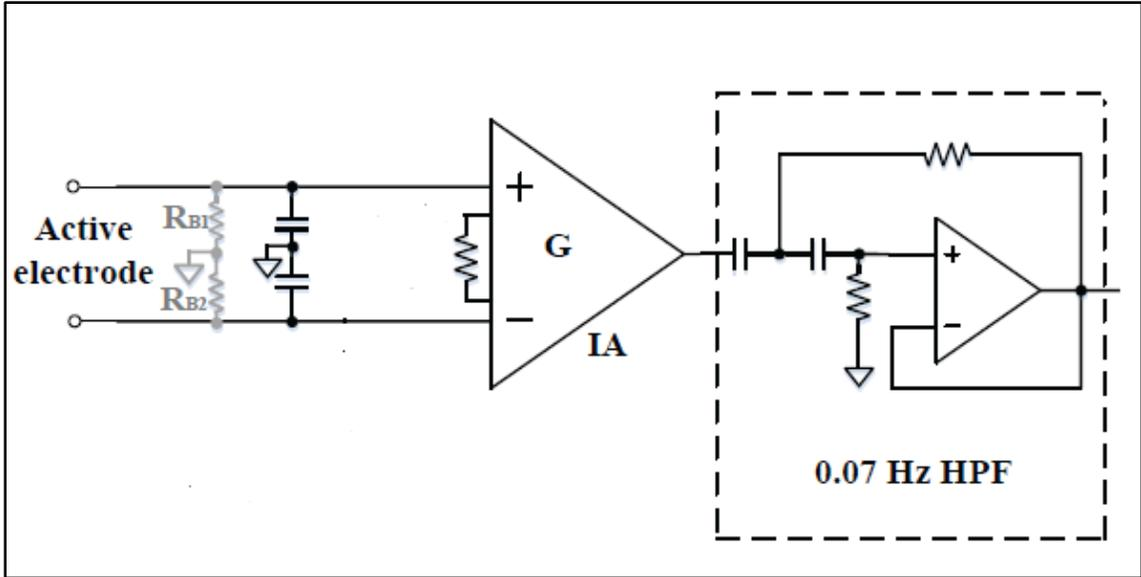
**Figure 6.3:** Schematic of the touch sensing device.
