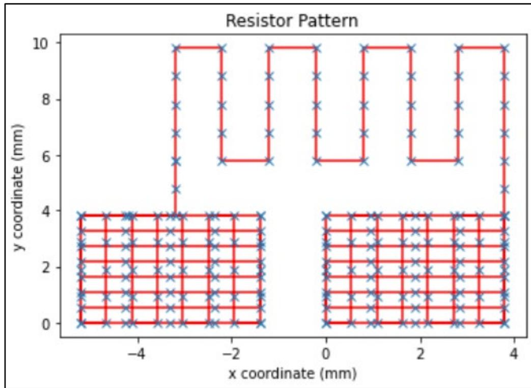
**Figure 4.1:** A resistor created with improper thread. The unit resistance of this thread was too low for the target resistance.
