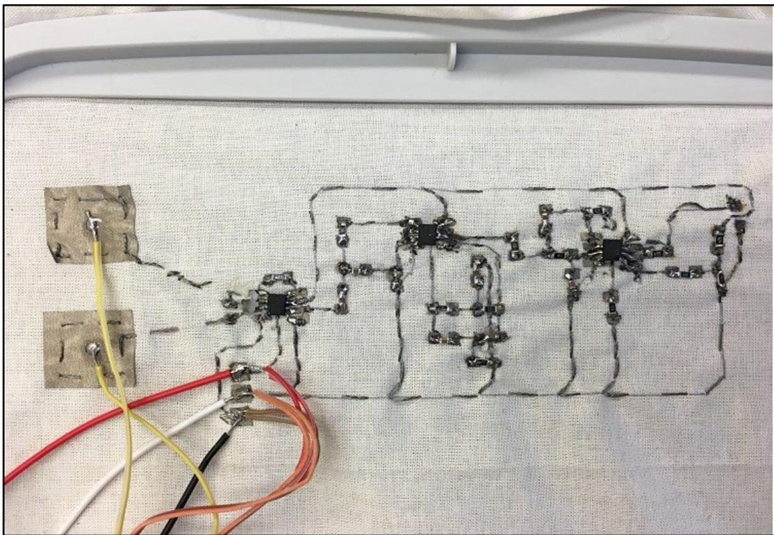
**Figure 1.3:** Wearable ECG detector with rigid resistors. Each rigid resistor needs to be soldered on and limits the flexibility of the device.
