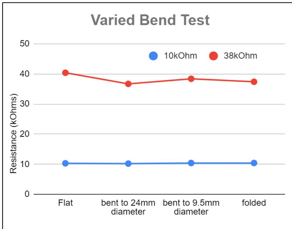
**Figure 5.2:** Varied bend consistency test
