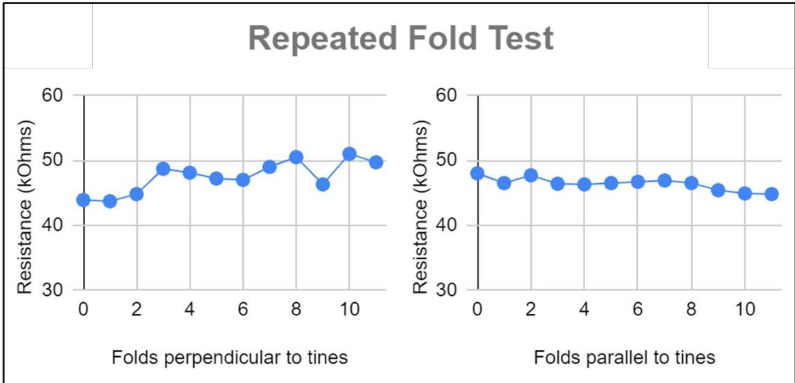
**Figure 5.5:** Repeated fold test to compare the effect of perpendicular and parallel folding on resistance.
