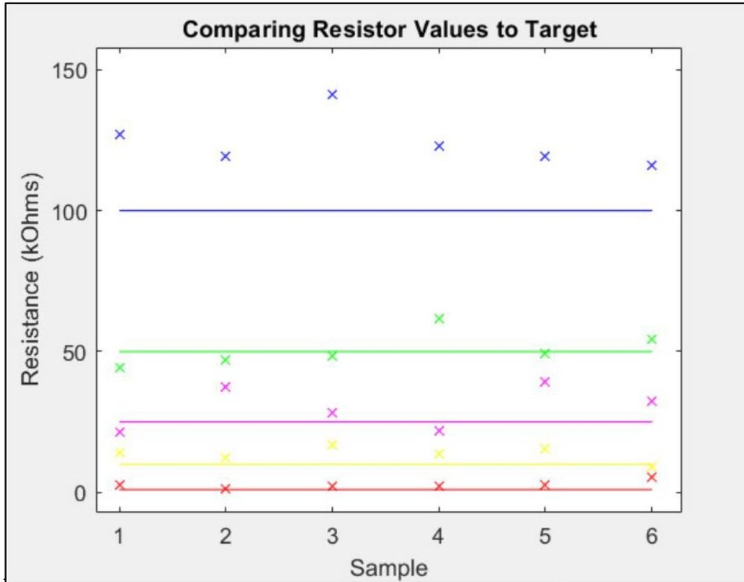
**Figure 5.8:** Batch Accuracy test to compare target and achieved resistances for 6 different strength resistors.
