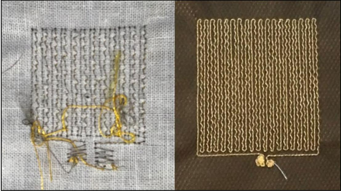
**Figure 4.7:** A comparison between a faulty Resistor with a short circuit (left) and a resistor with proper spaces (right).
