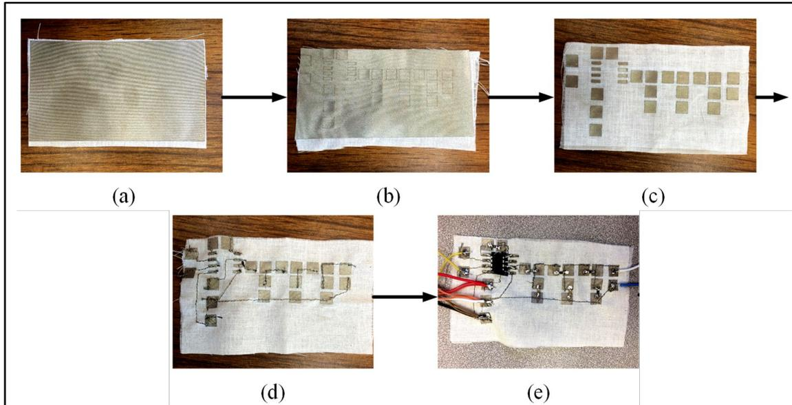
**Figure 6.2:** Manufacturing process for creating the touch sensing model with embroidery.
