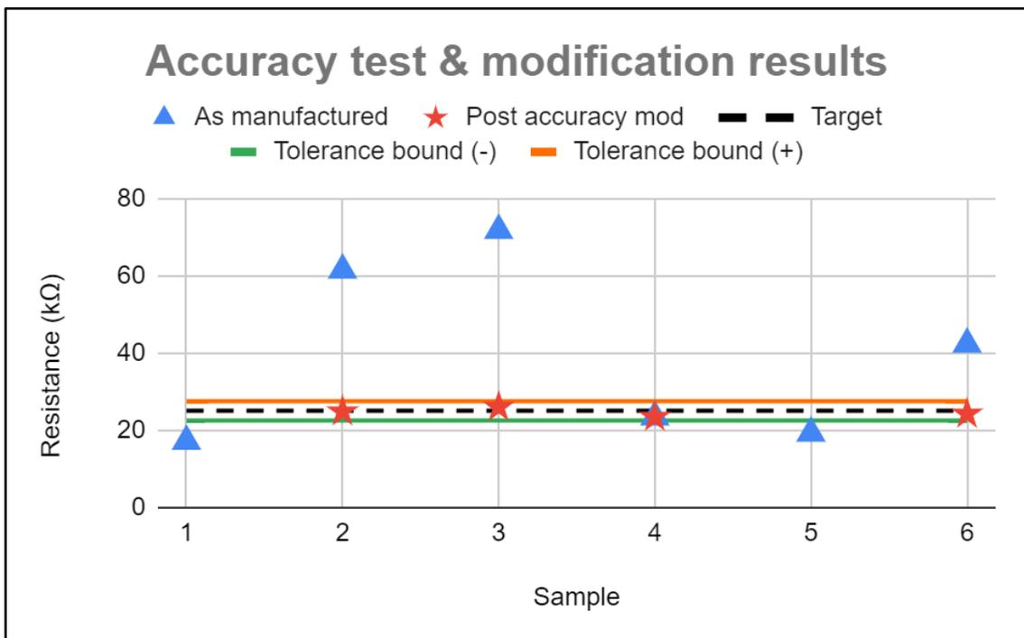
**Figure 5.9:** Batch accuracy test and the modification results.
