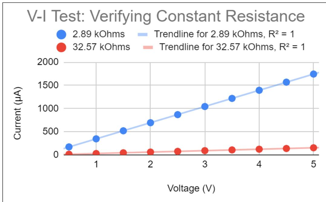
**Figure 5.1:** A VI (voltage-current) test
