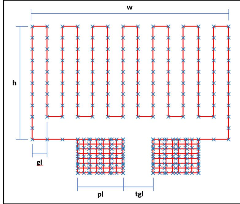
**Figure 3.2:** Parameters of resistor pattern. These parameters are the key measurements used by the RFGT in creating the resistor pattern and embroidery trace.
