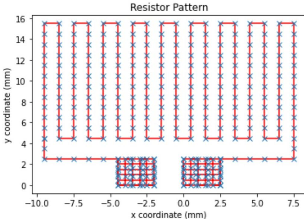
**Figure 3.1:** Depiction of the resistor design pattern with stitch locations.
