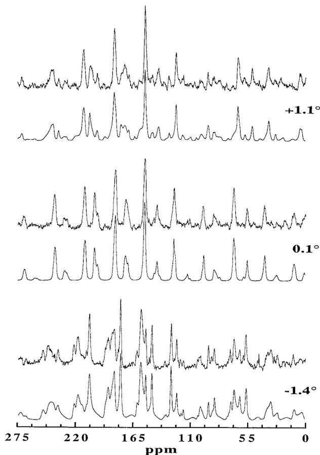
**FIG. 2.** Experimental  $^{13}\text{C}$  proton-decoupled, sample-spinning spectra and simulations for  $^{13}\text{C}$ -enriched  $\text{CH}_3^{13}\text{CN}$  at 140 K, spinning at 1100 Hz for three offsets from the magic angle. The parameters used for the simulations are a result of unweighted-least-squares fits. Values are discussed in the text.
