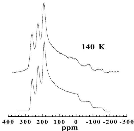
**FIG. 5.** Experimental  $^{13}\text{C}$  proton-decoupled spectra and simulation for  $^{13}\text{C}$ -enriched  $\text{CH}_3^{13}\text{CN}$ , for a stationary sample at 140 K obtained using Hahn echoes. The parameters used for the simulation are a result of unweighted-least-squares fits. Values are discussed in the text.
