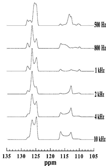
**FIG. 4.** Simulations of the zero-order sideband for  $\text{CH}_3\text{CN}$  spun at the magic angle for various spinning rates.
