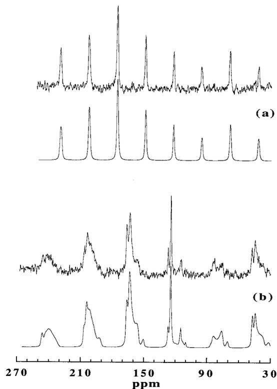
**FIG. 1.** Experimental  $^{13}\text{C}$  NMR proton-decoupled sample-spinning spectrum and simulations for  $^{15}\text{N}$ -enriched  $\text{CH}_3^{15}\text{N}$  at (a) the magic angle and (b) the magic angle minus  $1.8^\circ$ , at a spinning frequency of 1010 Hz. The methyl carbon signal is near 0 ppm and was not included in the simulation. The parameters used for the simulations are a result of unweighted-least-squares fits. Values are discussed in the text.
