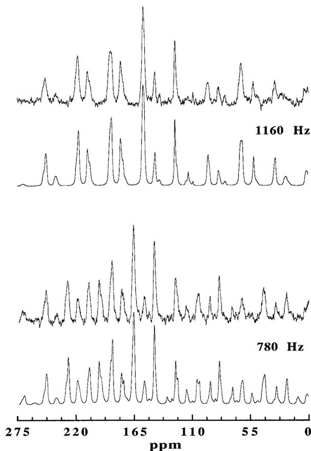
**FIG. 3.** Experimental  $^{13}\text{C}$  proton-decoupled, sample-spinning spectra and simulations for  $^{13}\text{C}$ -enriched  $\text{CH}_3^{13}\text{CN}$  at 180 K, and at the magic angle for different spinning rates. Spectra at spinning rates of 1160 and 920 Hz (not shown) were measured at both 140 K and 180 K and no difference could be observed. The parameters used for the simulations are a result of unweighted-least-squares fits. Values are discussed in the text.
