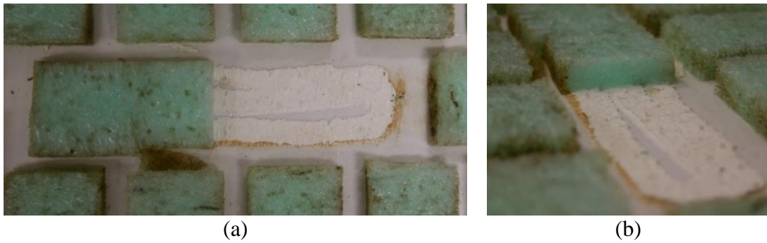
Figure 3.1. Cut away view showing adhesive underneath foam attached to c-Si-based flexible photovoltaic (PV) module: (a) top view and (b) orthogonal view.
