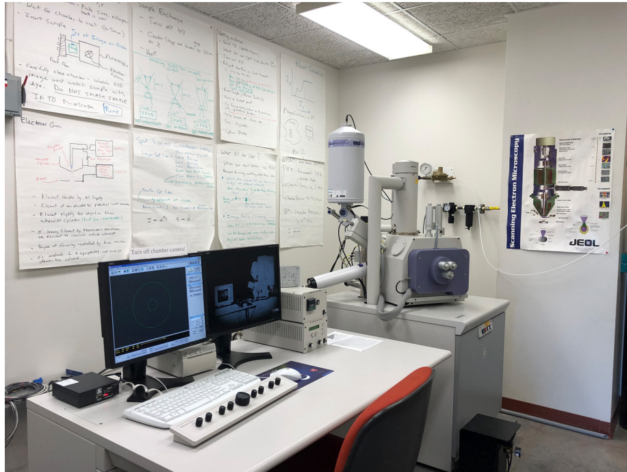
Figure 3.33 Philips/FEI XL30 ESEM used for the fracture surface analysis.
