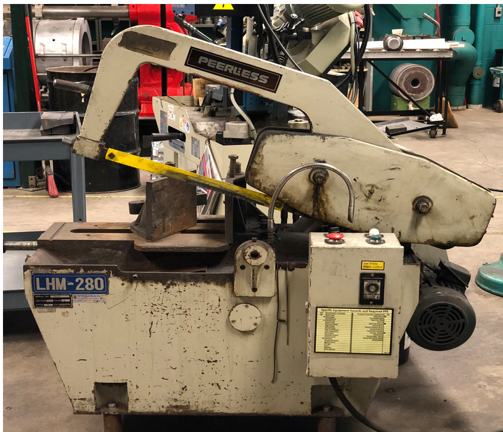
Figure 3.44 Hacksaw used to cut the 1-inch Y-blocks.
