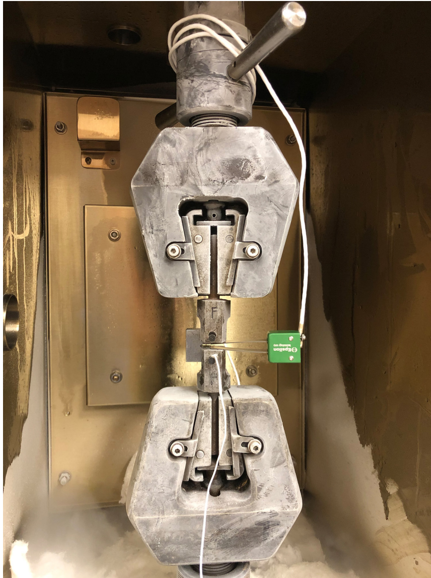
Figure 3.31 Assembly inside the cooling chamber at -20^{\circ}\text{C} .
