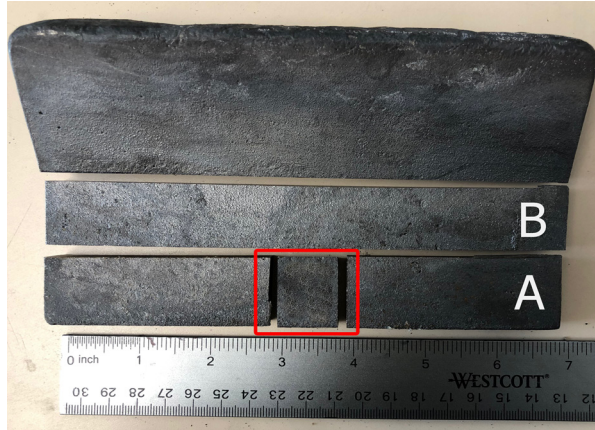
Figure 3.13 A and B bars showing the middle cross-section used for metallography per Y-block.
