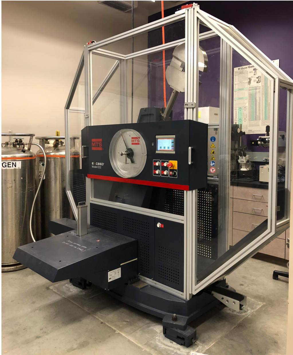
Figure 3.22 MTS Exceed® E22 impact test machine.
