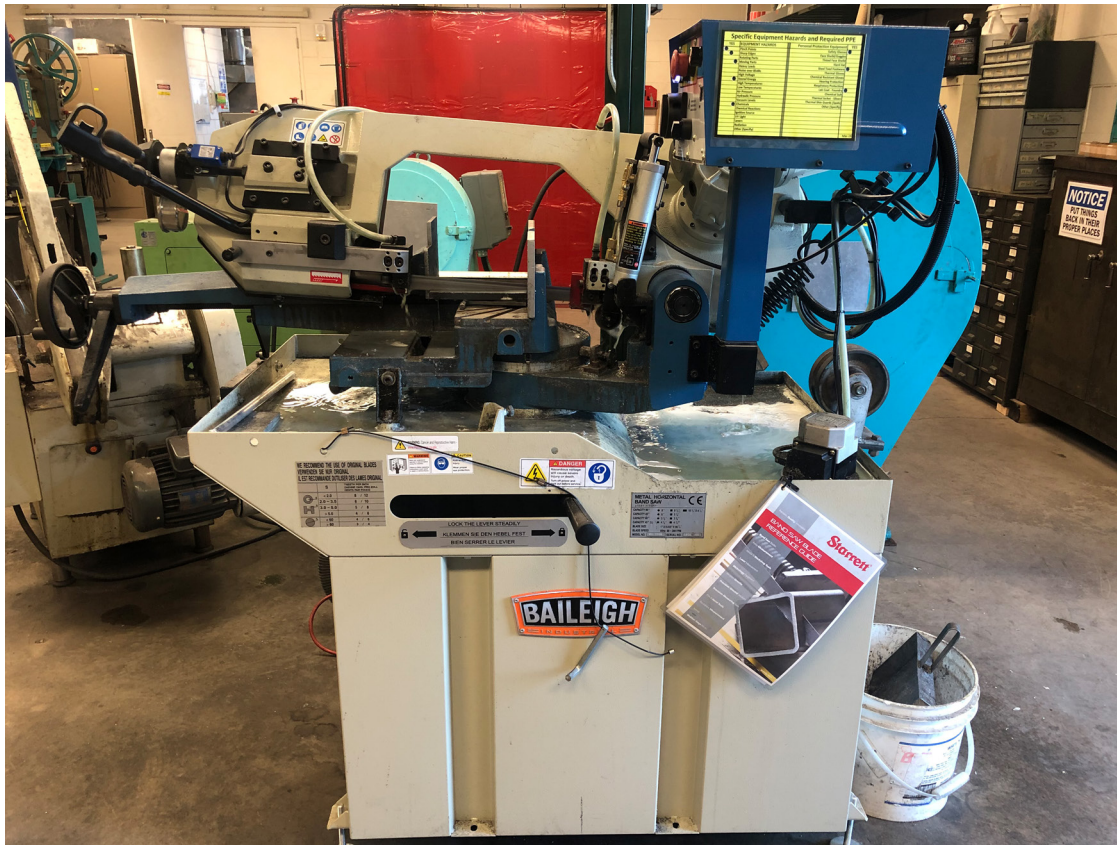
Figure 3.12 Band saw used to cut the ½ inch Y-blocks.
