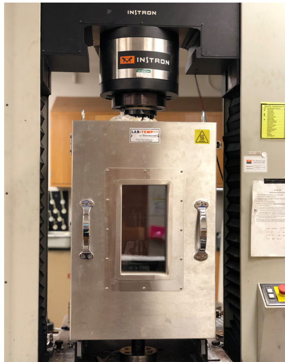
Figure 3.30 Portable LAB-TEMP™ furnace used for the low temperature testing.
