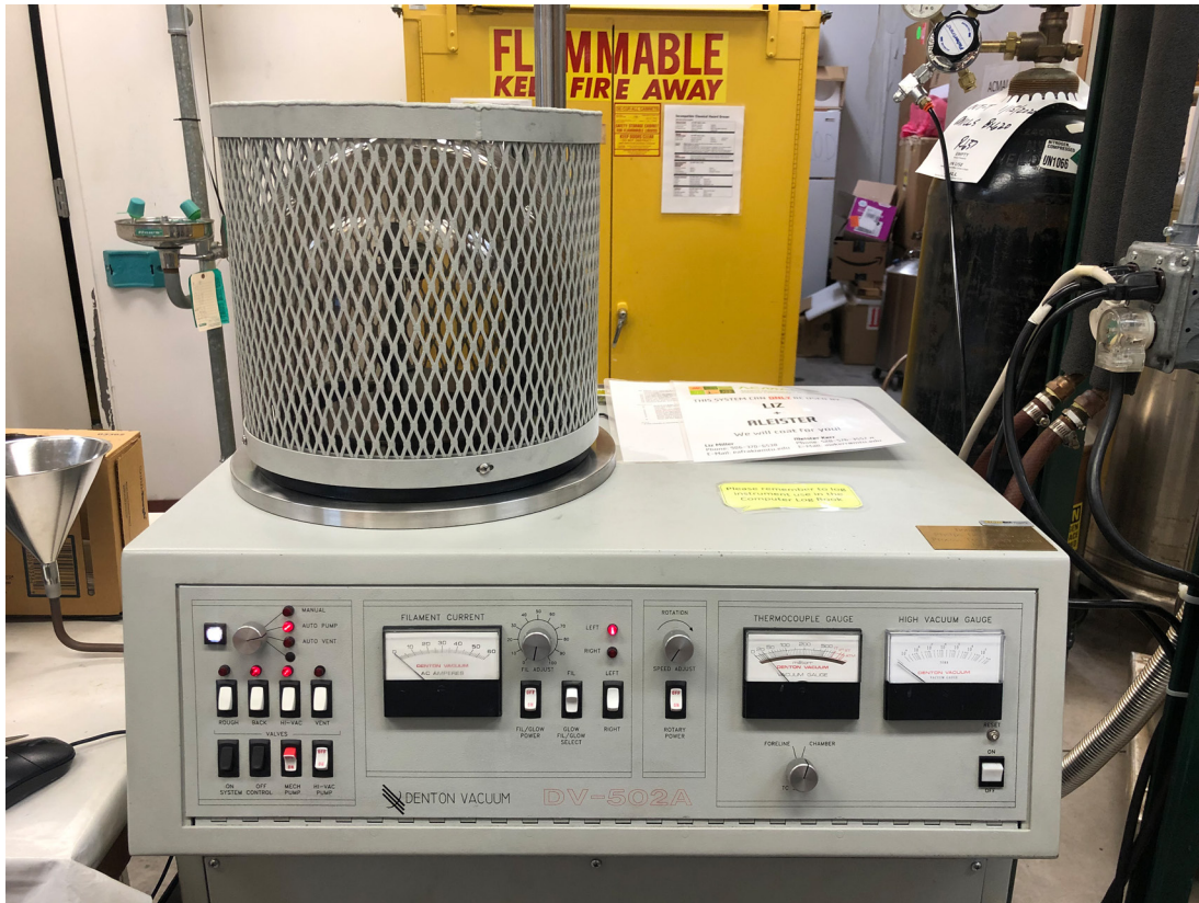
Figure 3.35 Denton DV-502A sputter coater used to carbon-coat the samples for EDS analysis.
