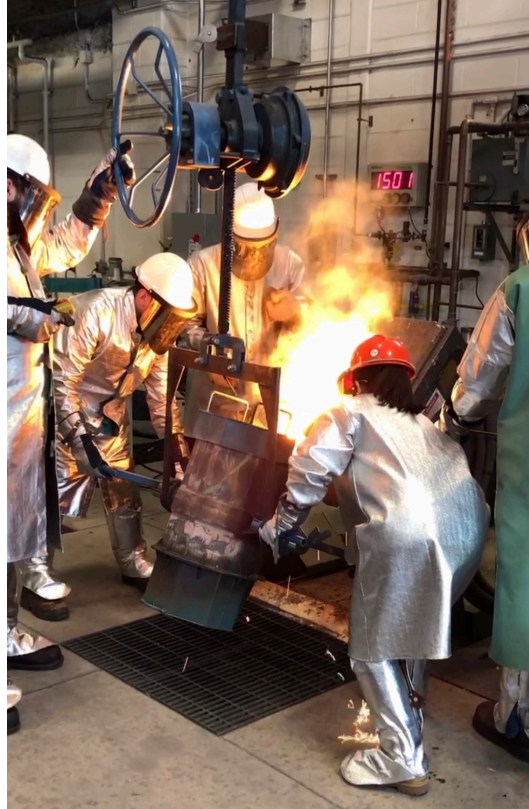
Figure 3.38 Tapping of the furnace to the tundish ladle.
