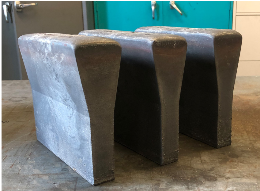
Figure 3.42 Set of three 1-inch Y-blocks after shaking out one mold.
