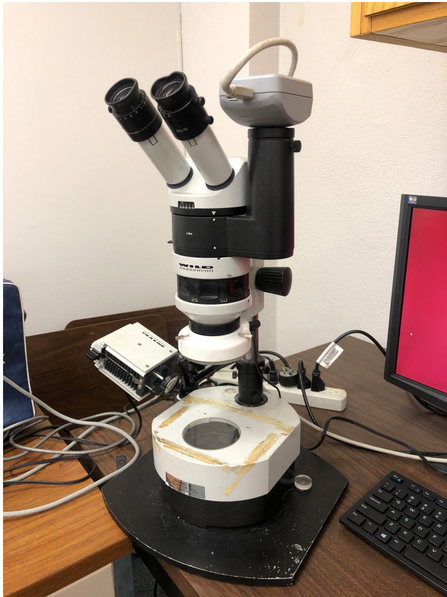
Figure 3.32 Wild Heerbrugg stereoscope used for analysis of the broken C(T) samples.
