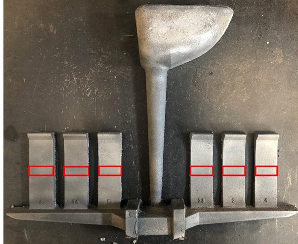
Figure 3.10 Location of the cross-section samples used for metallography.
