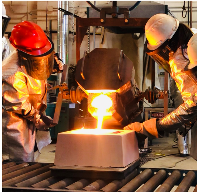
Figure 3.40 Pouring of one ASTM A536 1-inch Y-block mold.
