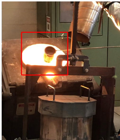
Figure 3.39 Metal stream inoculation using Inolate-40 enclosed in red.
