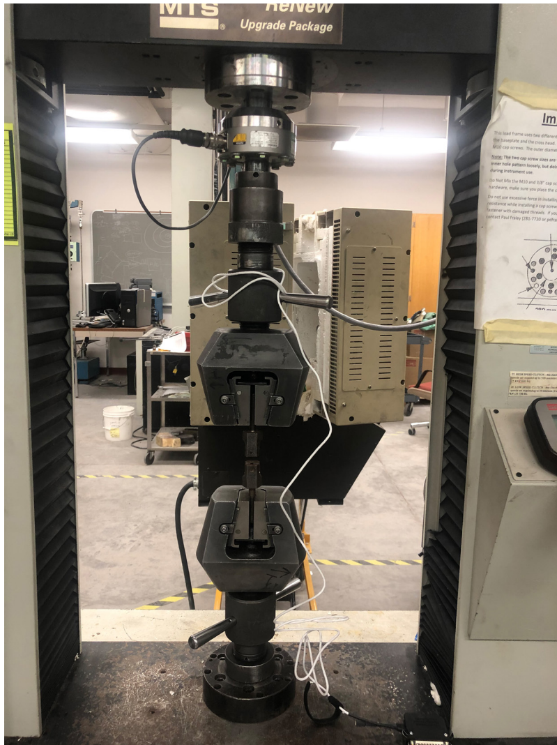
Figure 3.28 Instron 4206 machine used for the C(T) testing at room temperature.
