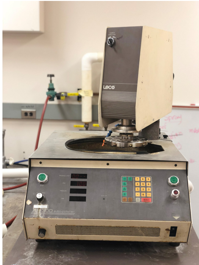
Figure 3.11 Leco AP-300 machine used for the metallographic preparation of the rectangular plates.
