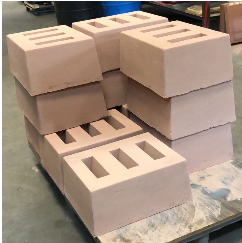
Figure 3.36 Chemically bonded 1-inch Y-block sand mold.
