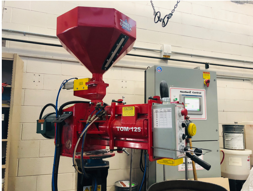
Figure 3.3 Tinker Omega NexGen2™ mixing system used to produce the chemically bonded sand molds.
