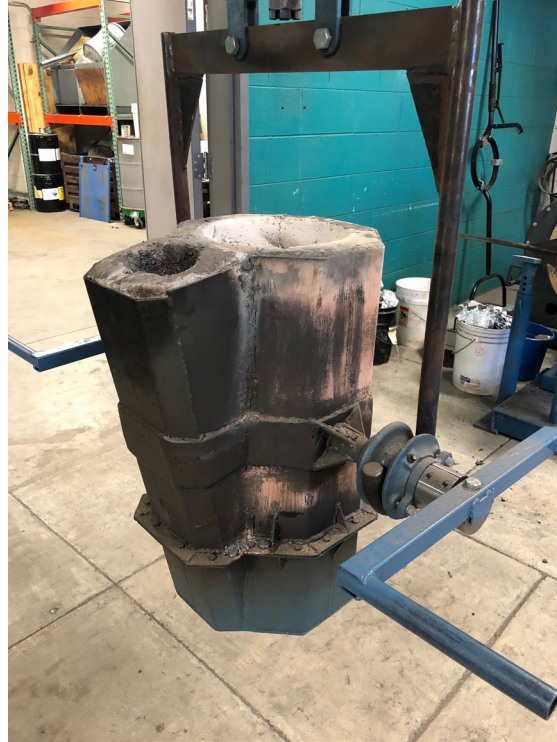
Figure 3.5 The 300-pound tundish ladle used for all the treatments.
