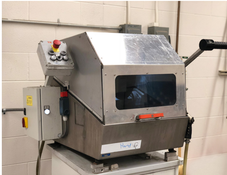
Figure 3.9 TR100 INOX LAPMASTER abrasive cutter used to cut the cross-sections for metallography of the rectangular plates.
