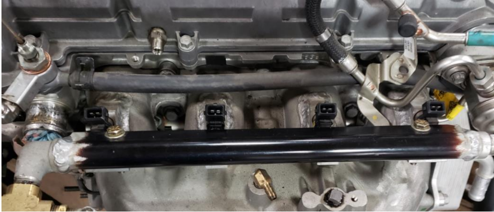
Figure 9 Water injection manifold, water rail and injectors
