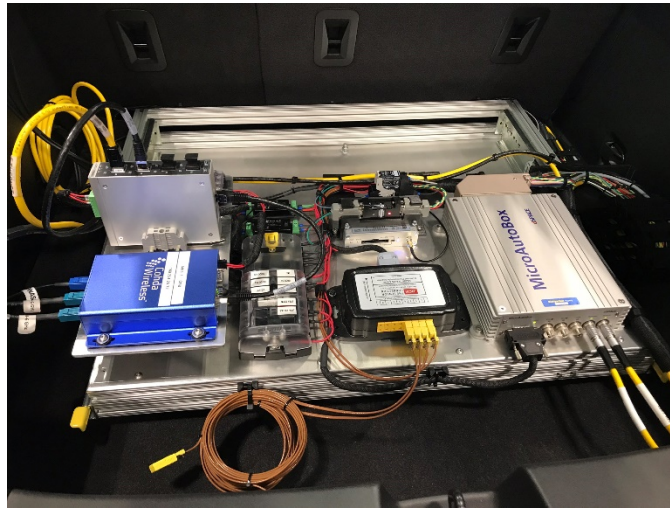
Figure 4-23: MTU Chevrolet Volt In-Vehicle Instrumentation Package.
