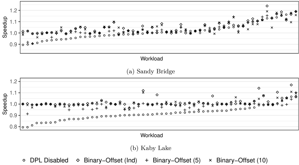
Figure 4.4: Workload performance for DPL prefetcher related policies on Sandy Bridge and Kaby Lake experimental environments, relative to baseline ALL ENABLED (all prefetchers enabled on all cores).
