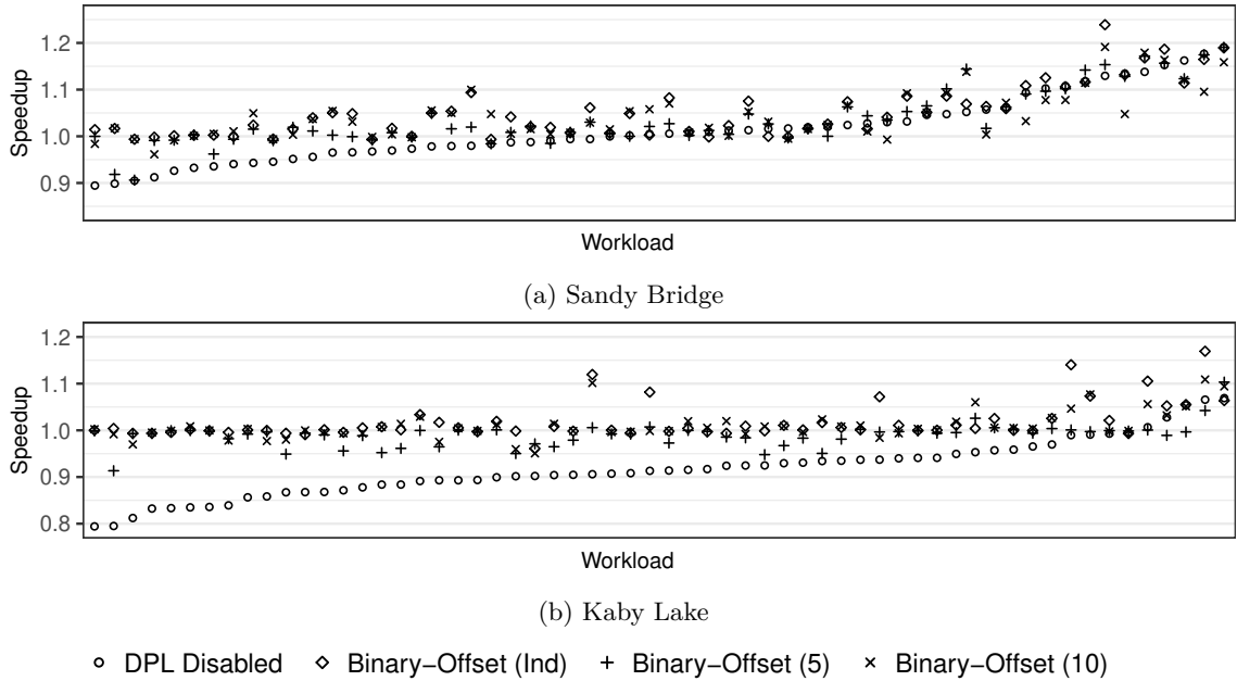
Figure 5.3: Workload performance for DPL prefetcher related policies on Sandy Bridge and Kaby Lake experimental environments, relative to the baseline.
