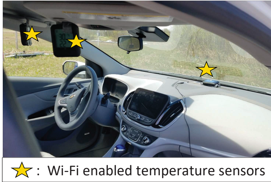
Figure 2.1: Test vehicle setup for solar load measurement at Keweenaw Research Center
