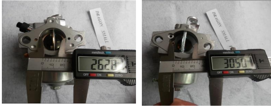
Figure 3.4: Base engine carburetor dimensions from online retailer
