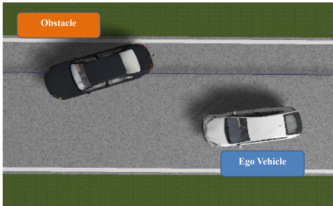
Figure 4.10: Ego vehicle deviating from the path to avoid collision with the obstacle
