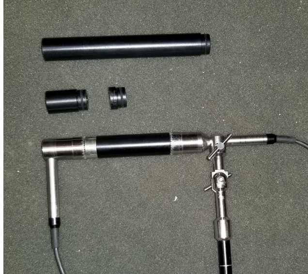
Figure 2-1. Face-to-face mic configuration with 1/2" mic and 50-mm spacer mounted on probe, and 12-mm, 25-mm and 100-mm spacers shown to the side
