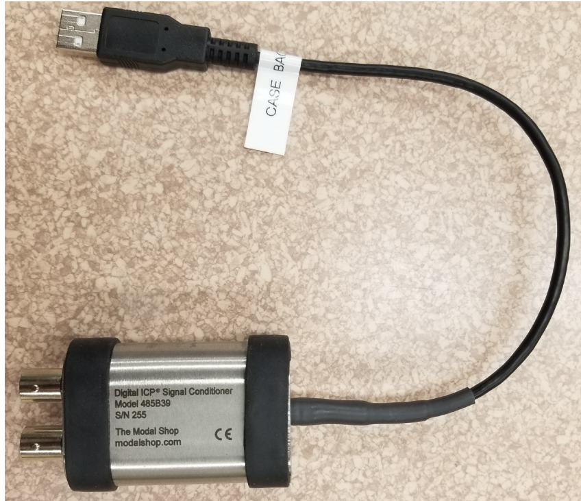
Figure 3-2. PCB 2-channel signal conditioner and A-to-D converter (Model 458B39)
