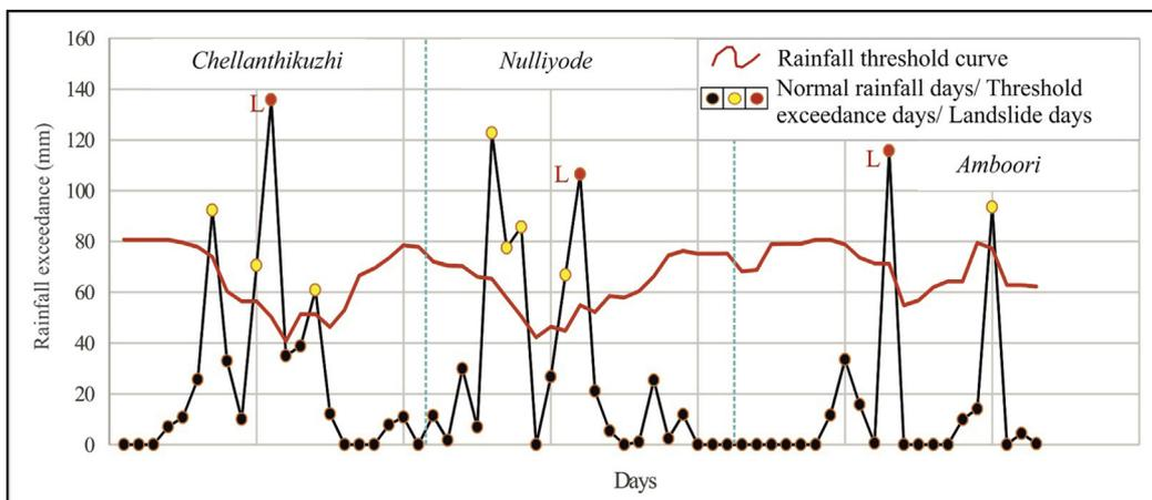
**Figure 6.** Threshold exceedance graph for 5-day antecedent vs. daily rainfall. 'L' indicates landslide incidence.
