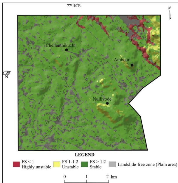
**Figure 8.** Slope stability units derived using the PISA-m model.
