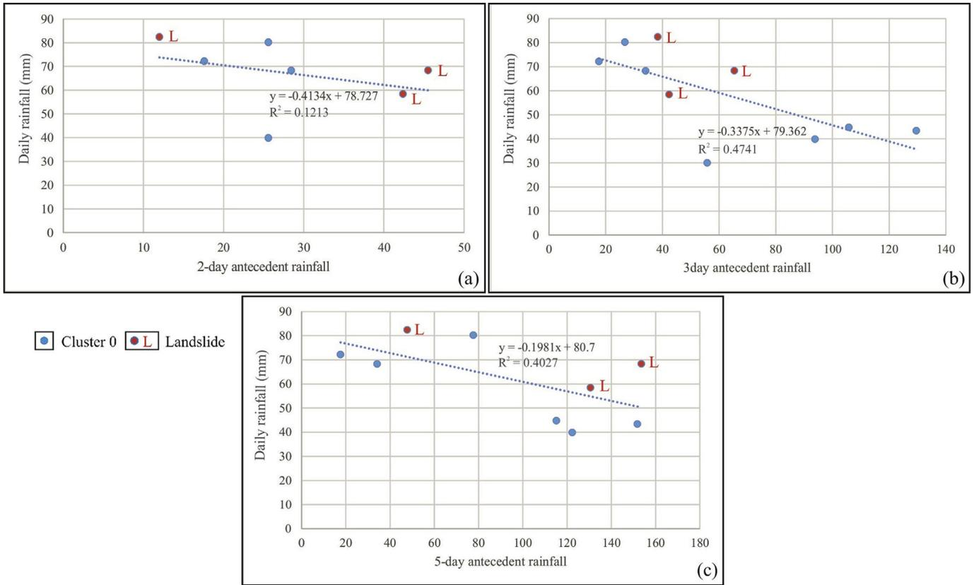
**Figure 5.** Linear trend line for isolated cluster favoring landslide. (a) 2-day antecedent vs. daily rainfall; (b) 3-day antecedent vs. daily rainfall; (c) 5-day antecedent vs. daily rainfall. 'L' indicates landslide incidence.
