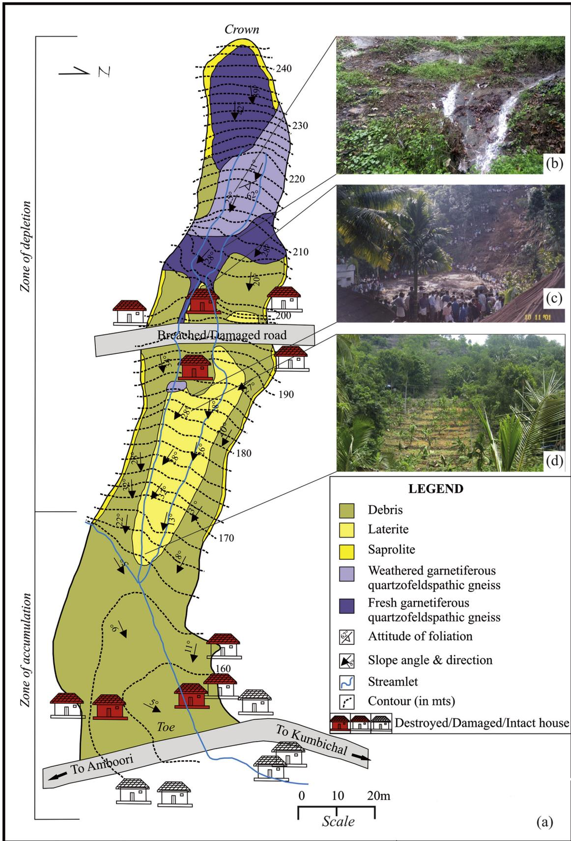
**Figure 3.** (a) Detailed site specific map of Amboori landslide prepared on 1:2000 scale (Source: [Muraleedharan and Sajinkumar, 2011a](#)); (b) removal of debris resulted in exposing rocky outcrops and water gushing through the landslide affected area. The flow is not confined to a channel; (c) rescue operations immediately after the landslide; (d) the landslide affected area has been stabilized by terrace cultivation.
