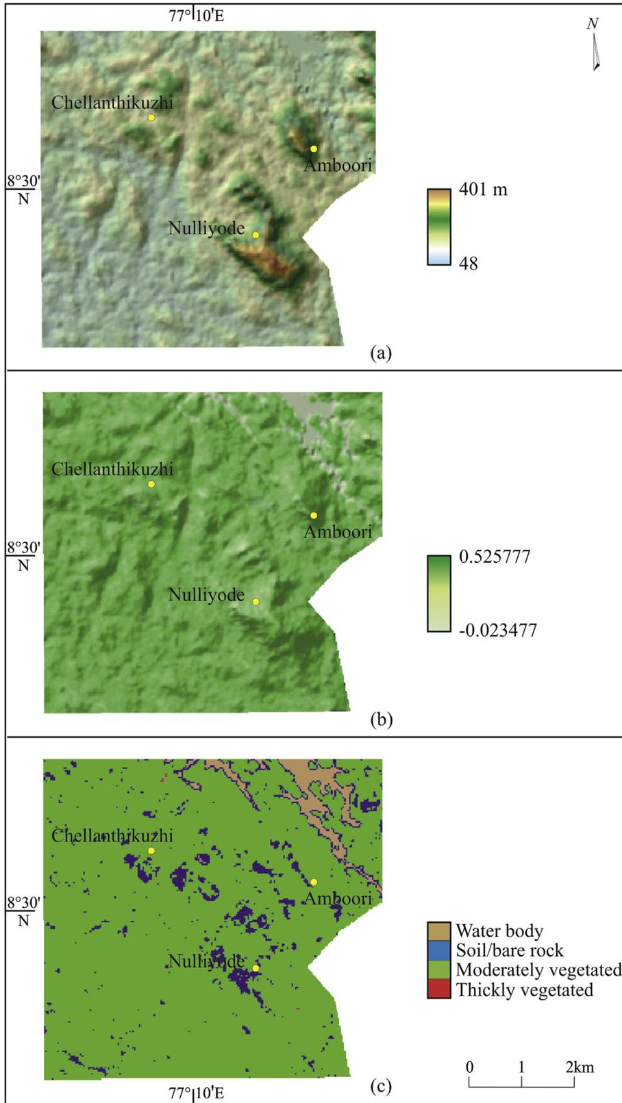
**Figure 7.** Thematic maps used in slope stability analysis using PISA-m. (a) DEM derived from 30 m resolution SRTM data; (b) NDVI derived from Landsat 8 imagery; (c) reclassified NDVI.
