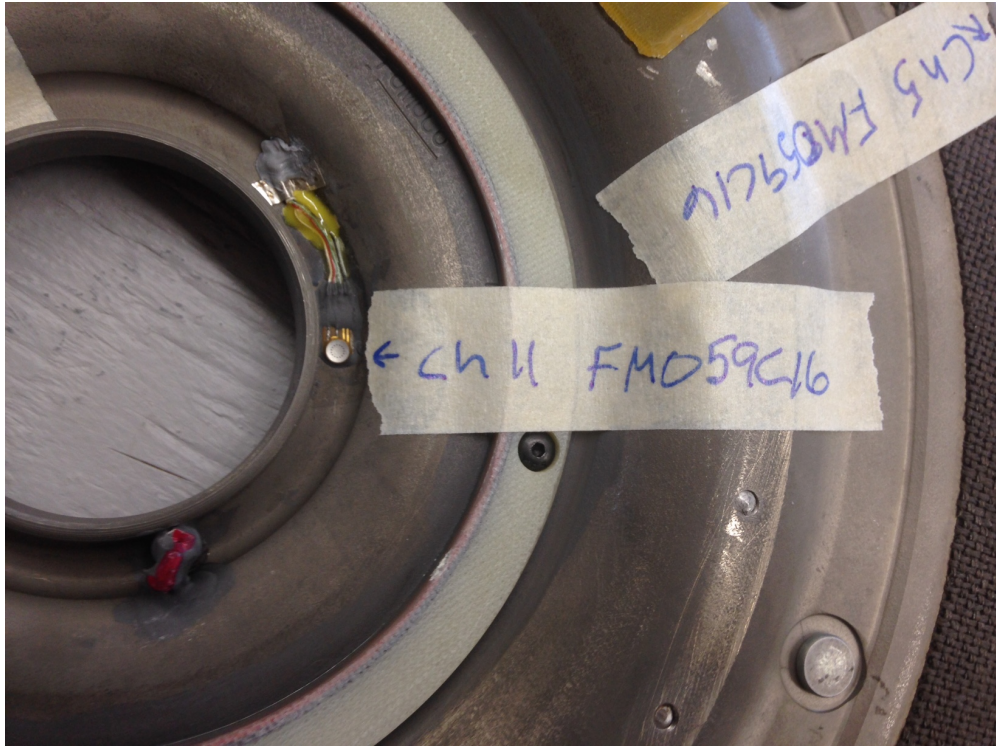
Figure I-43. Clutch channel 11 location, inner radius
