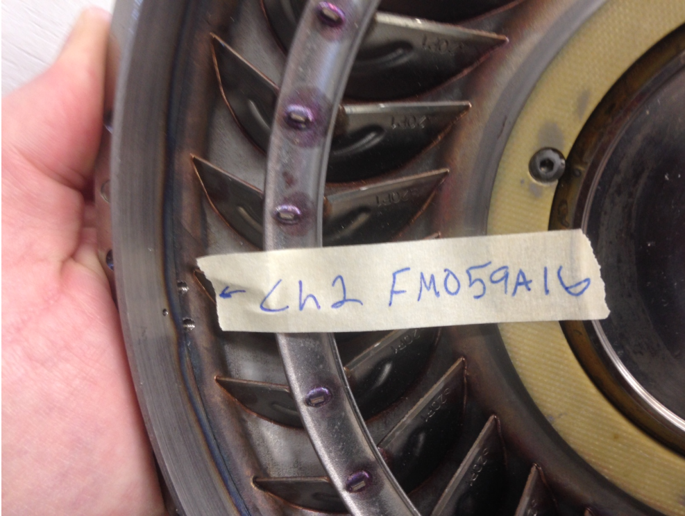
Figure I-17. Impeller channel 2 location, between impeller and turbine
