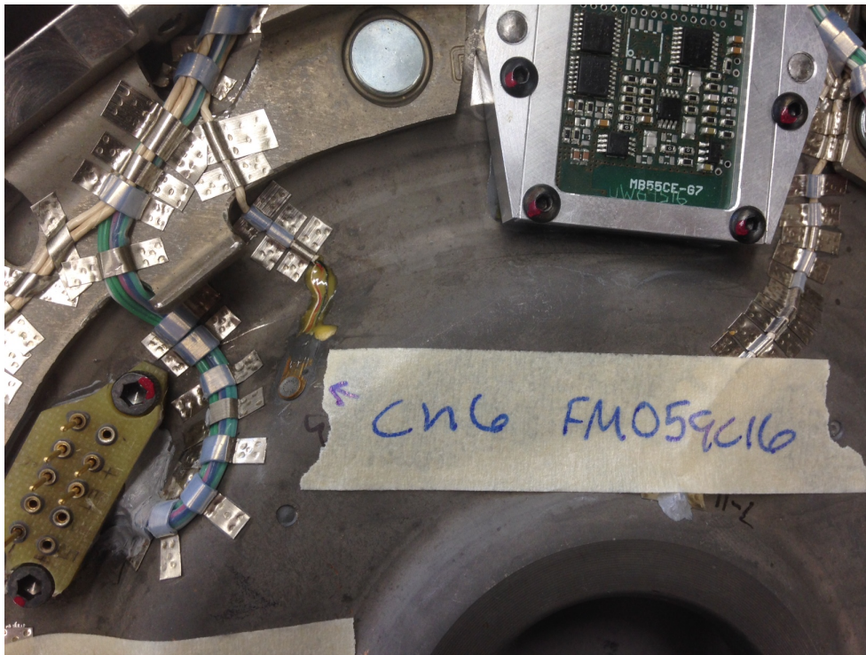
Figure I-45. Clutch channel 6 location, middle radius
