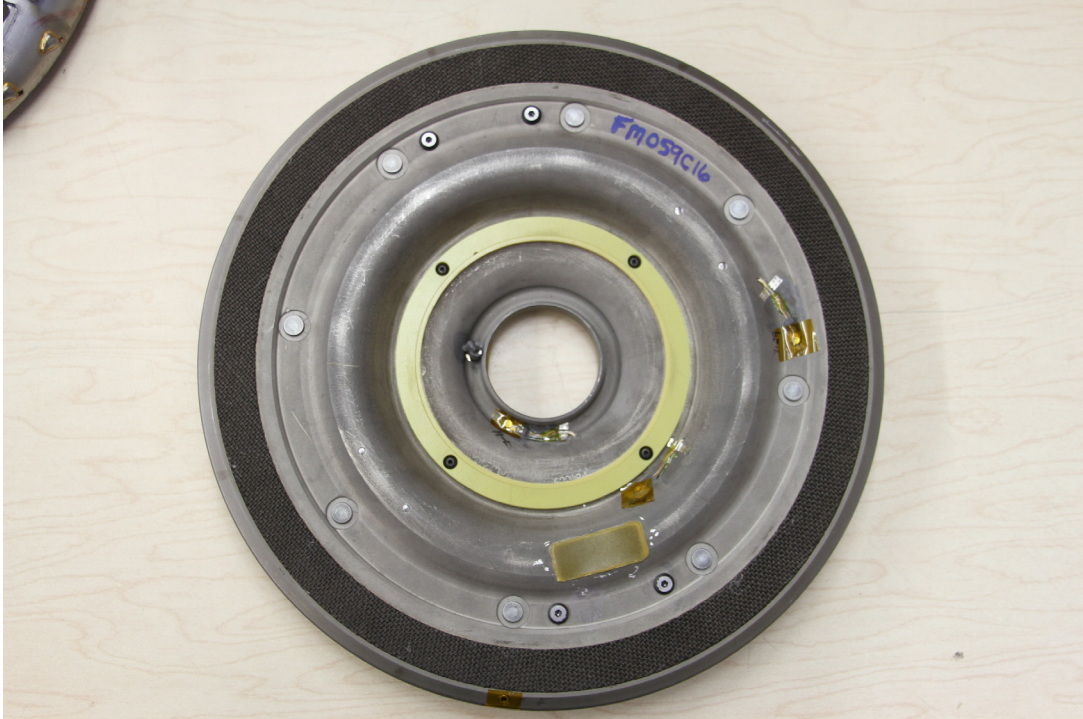
Figure I-5. Kevlar patch on clutch plate for transmitter
