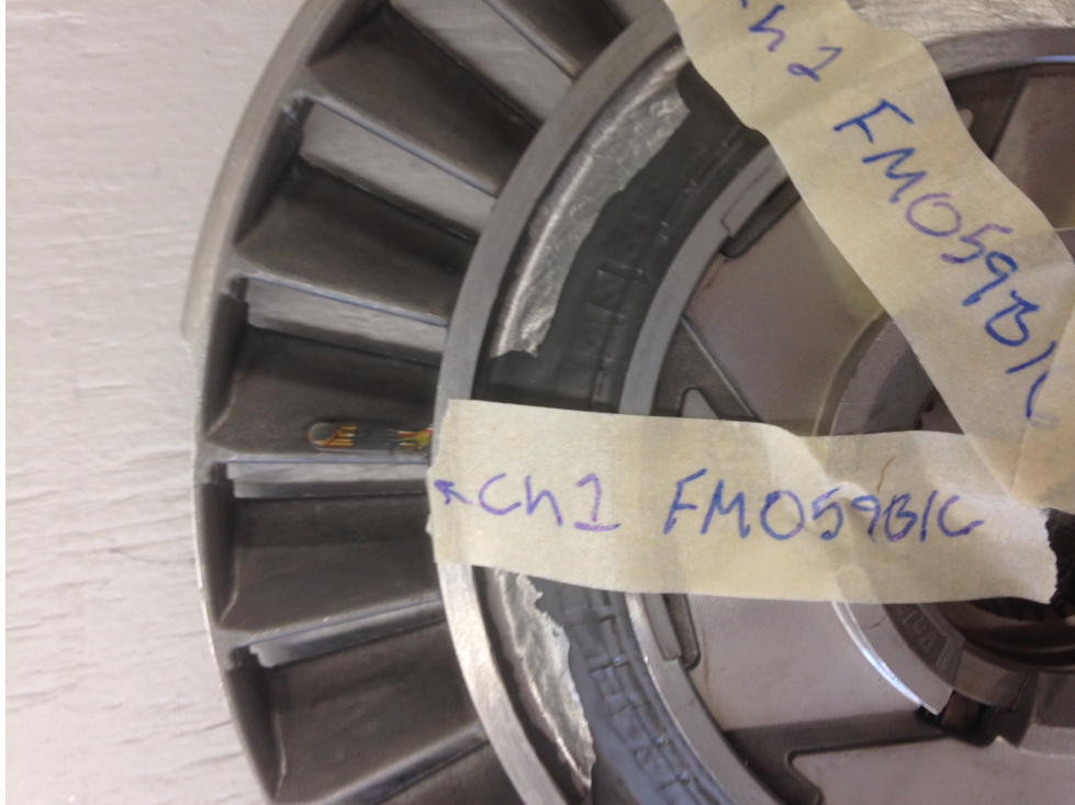
Figure I-23. Stator channel 1 location, leading edge/middle/pressure side
