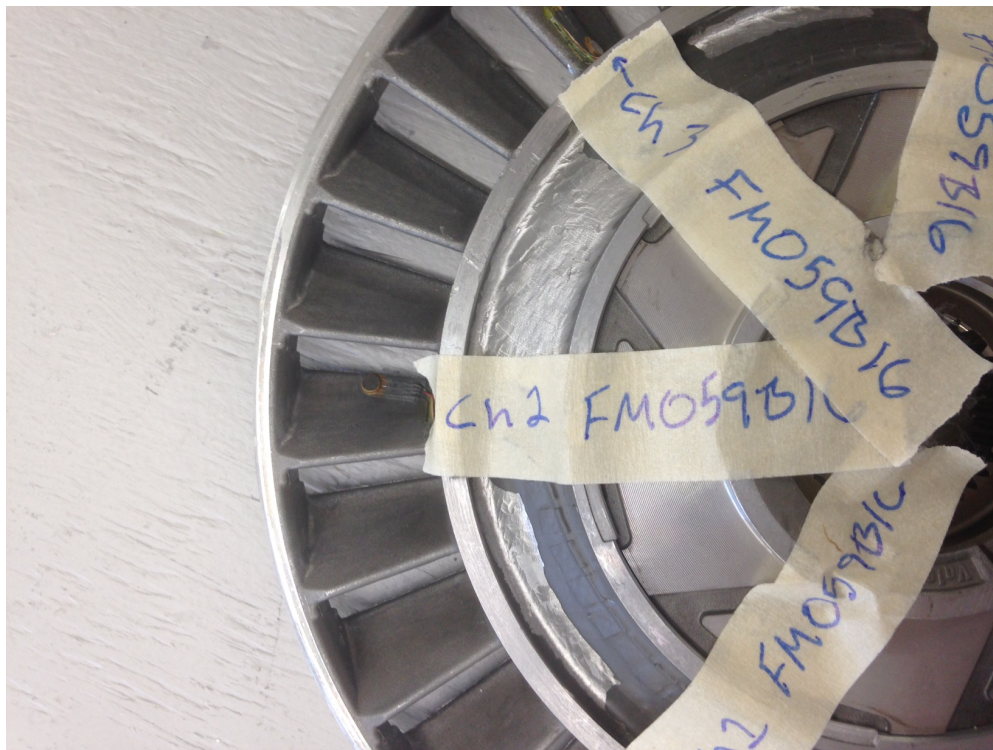
Figure I-24. Stator channel 2 location, trailing edge/middle/pressure side
