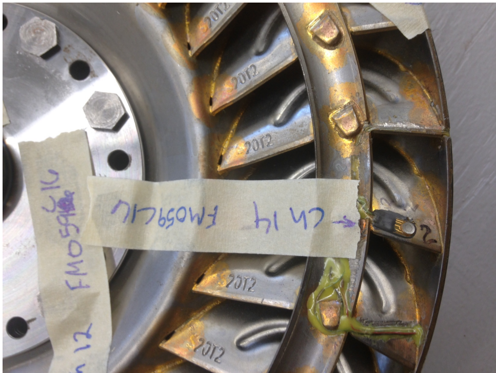
Figure I-36. Turbine channel 14 location, leading edge suction side
