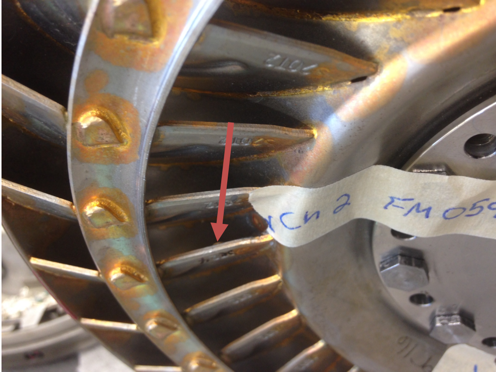
Figure I-33. Turbine channel 2 location, trailing edge pressure side
