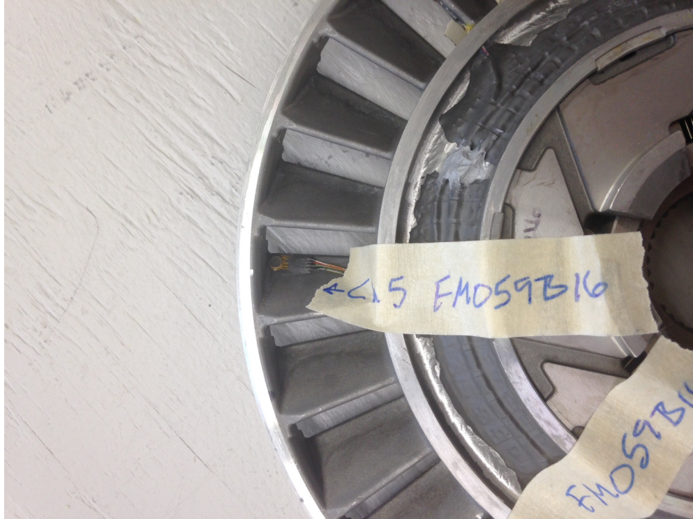
Figure I-27. Stator channel 5 location, trailing edge/shell/pressure side
