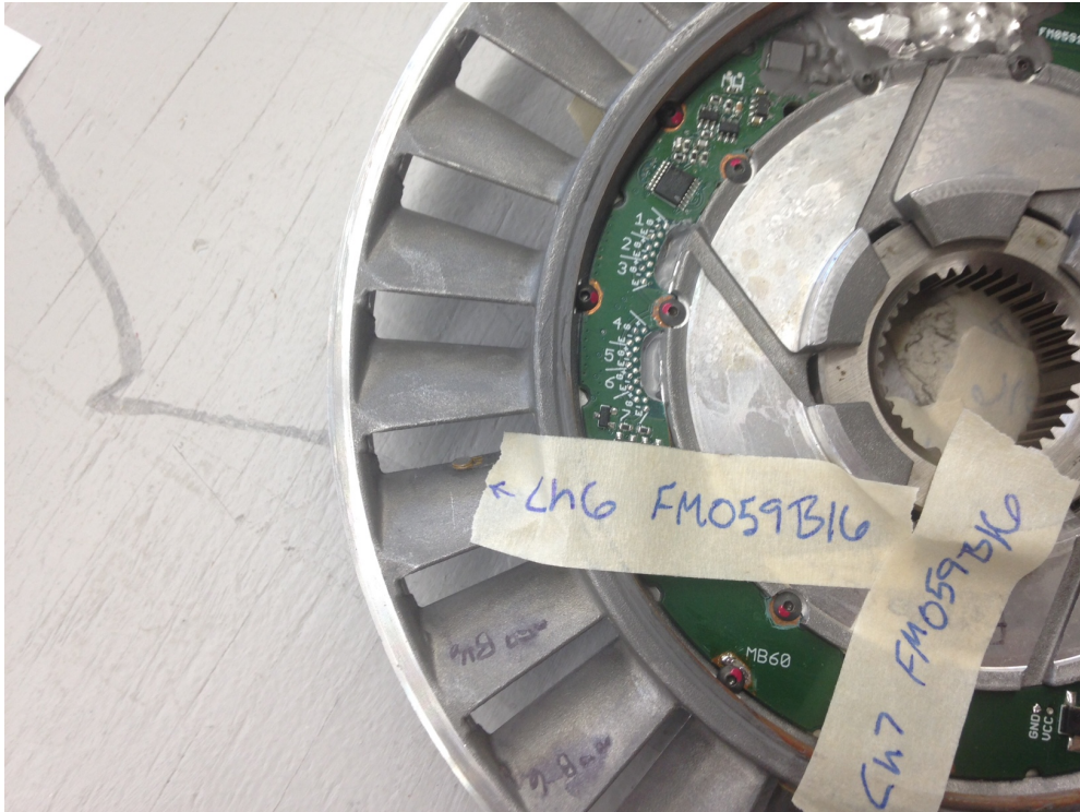
Figure I-29. Stator channel 6 location, leading edge/middle/suction side
