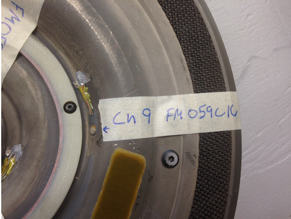
Figure I-41. Clutch channel 9 location, middle radius
