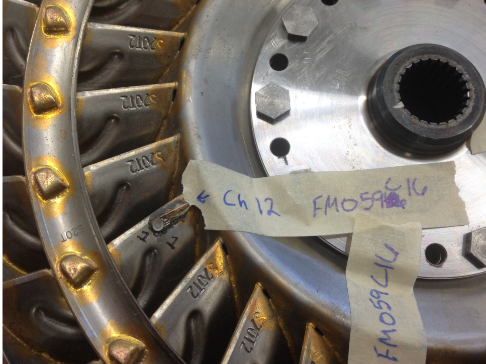
Figure I-35. Turbine channel 12 locations, trailing edge suction side
