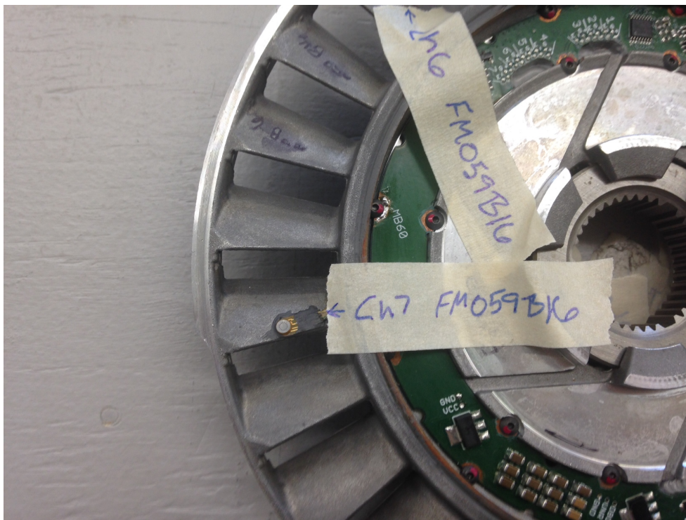
Figure I-30. Stator channel 7 location, trailing edge/middle/suction side
