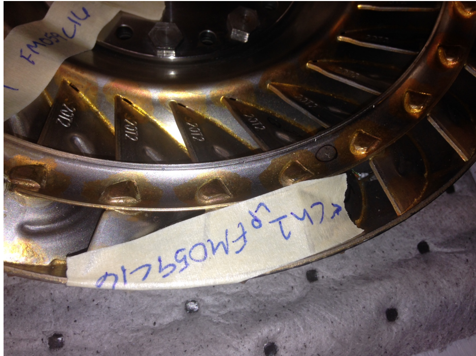
Figure I-32. Turbine channel 1 location, middle of blade suction side
