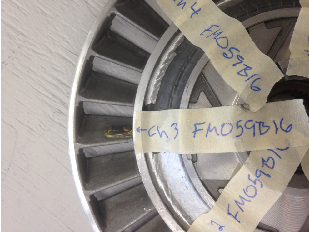
Figure I-25. Stator channel 3 location, middle of blade/shell/pressure side
