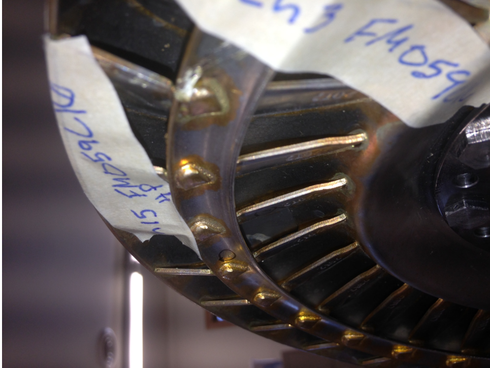
Figure I-37. Turbine channel 15 location, middle blade pressure side
