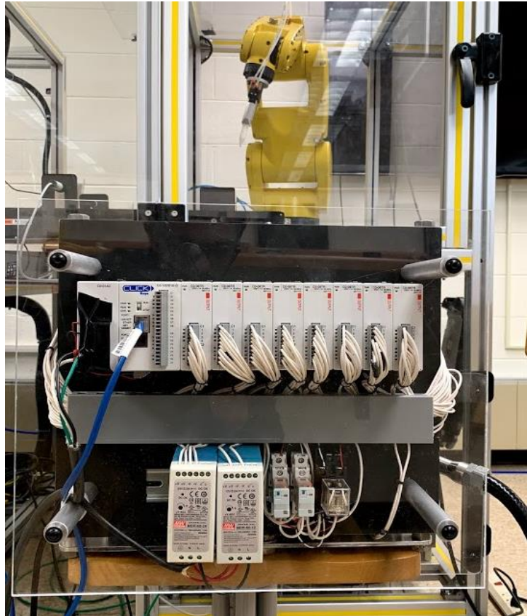
Figure 2: The final setup of remote robot system with FANUC LR-Mate 200iC robot and CLICK PLC
