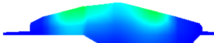
Figure 4-107. Predicted equivalence ratio distribution for injection timing -45 deg ATDC for charge pressure a) 1.41 Bar at 8 deg ATDC and b) 2.41 Bar at -6 deg ATDC
