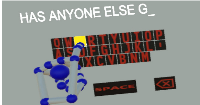
Figure 3.1: A left handed participant entering text on the virtual keyboard in the UNIMANUAL condition. When the participant touches a key it is highlighted yellow. When he takes the finger off the keyboard surface, it is added to the observation and shown in the display.
