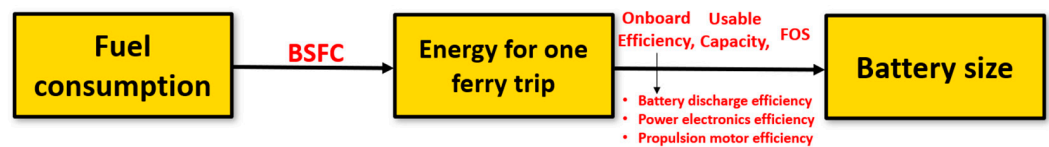
Figure 7. Schematic of the battery sizing process.
