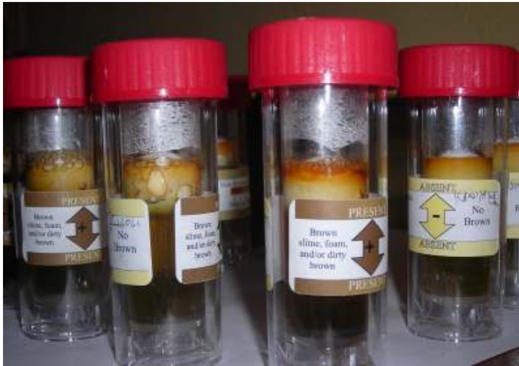
Figure 4.2 From left to right: bubbles appearing in IRB-BART™ samples taken from Bukumi, Kigoli, and Bulegete. No bubbles in Kanyawawa’s sample. (photograph by author)
