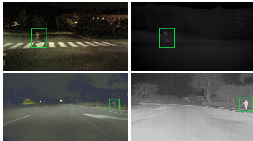
Figure 1. (Left column): The visual images from the KAIST and FLIR datasets provide distinctive visual features; however, in low lighting, human silhouettes are more apparent in the infrared domain (Right column).
