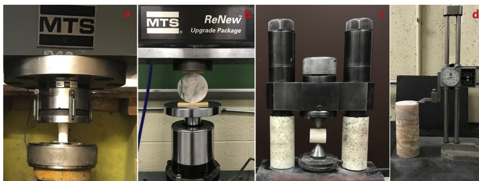
Fig. 2. Apparatuses used in the laboratory for (a) UCS, (b) BTS, (c) PLI, and (d) parallelism measurement.
