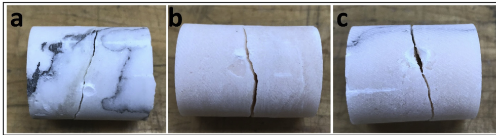
Fig. 18. Failure modes in PLI tests on samples with discontinuities situated at different directions, in respect to the applied point load (sample b with no apparent discontinuity).
