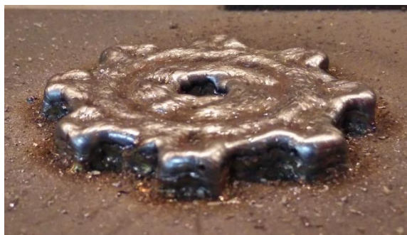
Figure 3.14 3 layers of 3-D printed gear (60 mm diameter).
