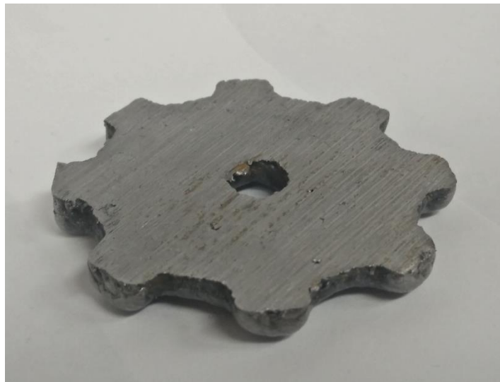
Figure 3.16 The finished machined gear (60 mm diameter).
