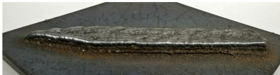
Figure 3.13 3 layers of 3-D printed chisel (140 mm × 20 mm × 20 mm).
