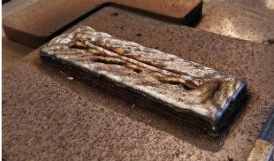
Figure 3.11 Poor surface quality after third layer of printing speed 10 mm/s on block (101.6 mm × 31.75 mm).
