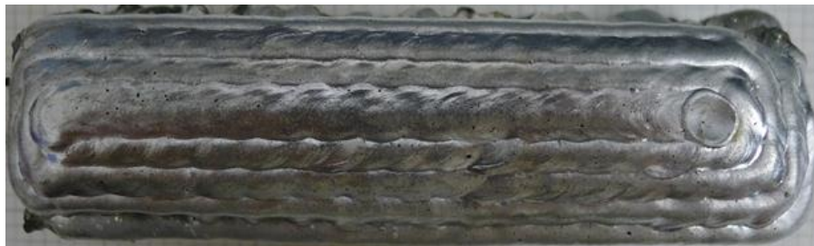
Figure 2.7 Example top surface of a 4943 printed specimen viewed in the direction of the z-axis.
