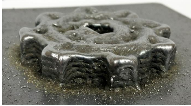
Figure 3.15 The finished 3-D printed gear (60 mm diameter) (5 layers).
