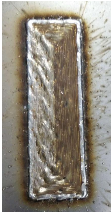
Figure 3.17 With optimal settings, brown oxide due to one side blocked shield gas (101.6 mm × 31.75 mm).
