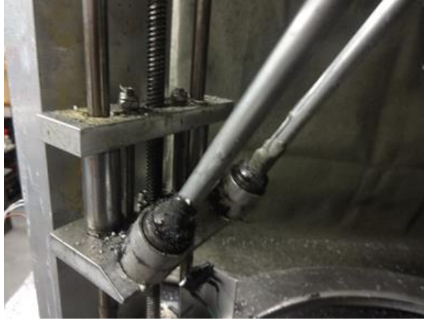
Figure 2.2 Detail of carriage assembly and magnetic ball joint with sleeves on the open source metal RepRap 3-D printer. The lead screw from the stepper motor driving that carriage is also visible in the center of the image.
