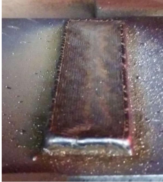
Figure 3.12 3 layers of 3-D printed block (101.6 mm × 31.75 mm).
