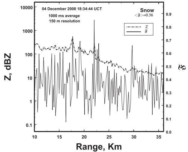
FIG. 2. As in Fig. 1, but for a different snow event and the resolution is only 150 m. The corresponding smaller value of  $\langle \varrho \rangle$  is likely due to enhanced decorrelation over a sample volume 20 times greater than in Fig. 1.
