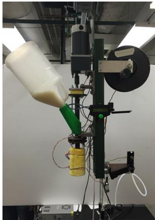
Figure 3. Vertical recyclebot. The white hopper is on the upper left and the black spooler is on the upper right. The motor in the upper middle drives an auger that feeds plastic into the hot zone (insulated in yellow). Filament is produced and looped through a light sensor to maintain the loop length, and thus the filament diameter, automatically. In this setup, the length and diameter can be measured continually.
