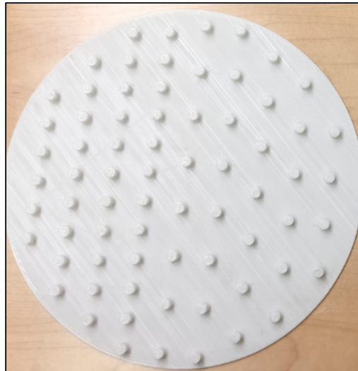
Figure 7. Dimpled mat 3-D printed with NinjaFlex. The spacing of the dimples can be adjusted to hold various tube sizes.
