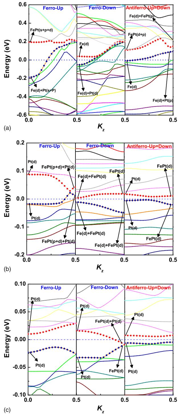
FIG. 5. (Color online) Spin-polarized energy-band structures: (a) two-spacer; (b) five-spacer; (c) eight-spacer layer nanowires. The Fermi energy is set at  $E=0$ . Notations: gray (red) circle, conduction band; gray (blue) diamond, valence band.
