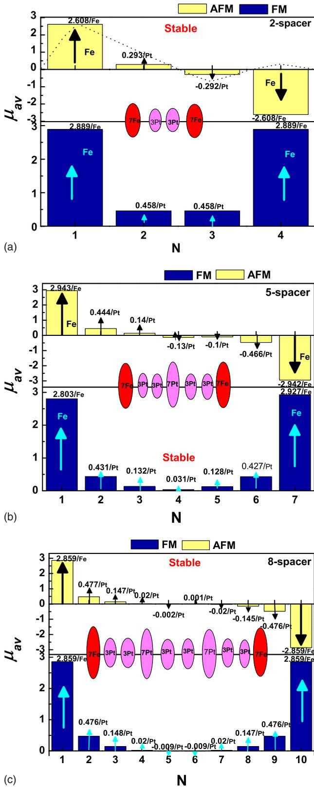
FIG. 4. (Color online) Histogram plot for the average magnetic moment per atom ( $\mu_{av}$ ) in FM and AFM configurations. (a) Two Pt spacer; (b) five Pt spacer; and (c) eight Pt spacer nanowires. Notations: dark gray (blue), FM; light gray (yellow), AFM; N is the layer number; dotted line in (a) represents RKKY type magnetic perturbation.
