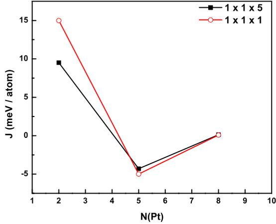
FIG. 3. (Color online) Calculated interlayer exchange coupling ( $J$ ) as a function of number of nonmagnetic Pt spacer layers  $N(\text{Pt})$  in the nanowire structures.  $1 \times 1 \times 1$  and  $1 \times 1 \times 5$  represent the  $k$ -point sampling of the BZ used to obtain the respective results.
