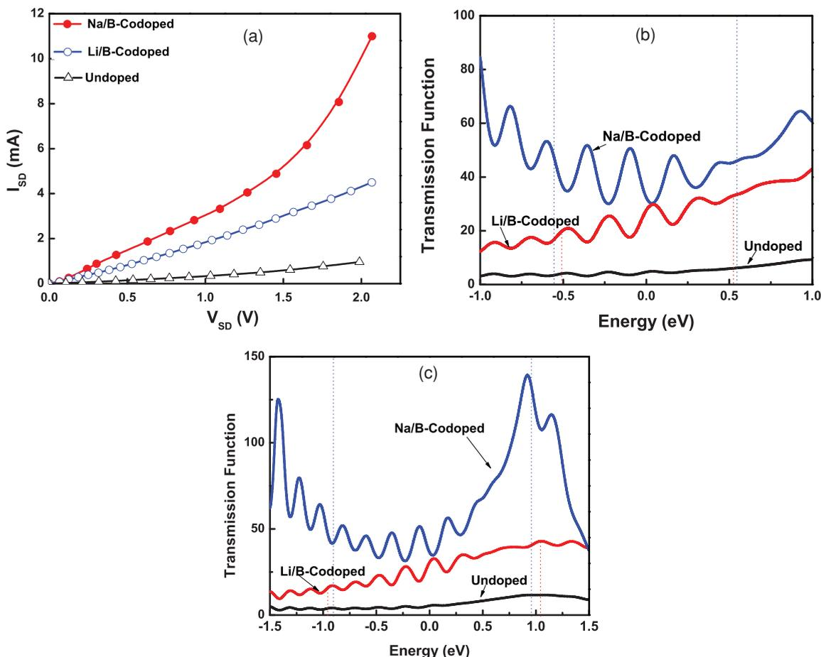
FIG. 3. (Color online) (a) Current-voltage characteristic of undoped junctions and junctions codoped with Li and B and with Na and B. (b) Bias-dependent transmission as a function of injection energy at (b)  $\sim 1$  V and (c)  $\sim 2$  V. The Fermi energy is set to zero in the energy scale and the dotted lines represent the chemical-potential window.
