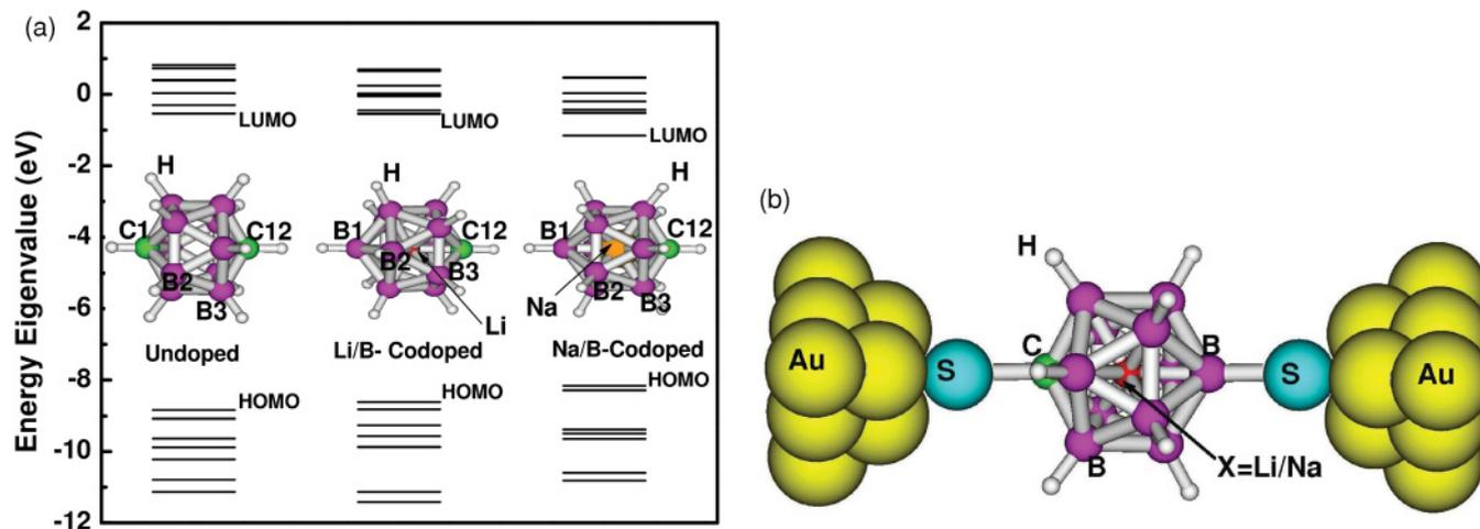
FIG. 1. (Color online) (a) Energy eigenvalues of  $C_2B_{10}H_{12}$ ,  $Li@C_1B_{11}H_{12}$ , and  $Na@C_1B_{11}H_{12}$ . Respective optimized structures are shown in the inset. (b) Schematic representation of alkali ( $X = Li, Na$ ) carborane junction codoped with B.
