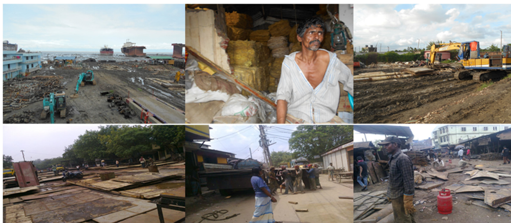
Figure 1. Shipbreaking yard with grab (top left), glasswool shop in Bhatiraty (top middle), magnetic grab carrying small sections for loading (top right). Shipbreaking scrap business in Dhaka city (bottom left), workers carrying plate in shoulder in Dhaka city (bottom middle), Cutters working in Dhaka city (bottom right). Photo Credit: First author, 14 June 2014.
