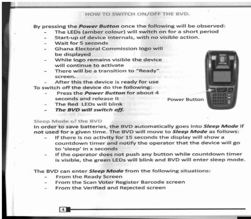
Figure 4.6: Instructions on how to switch device on/off.<sup>10</sup>
