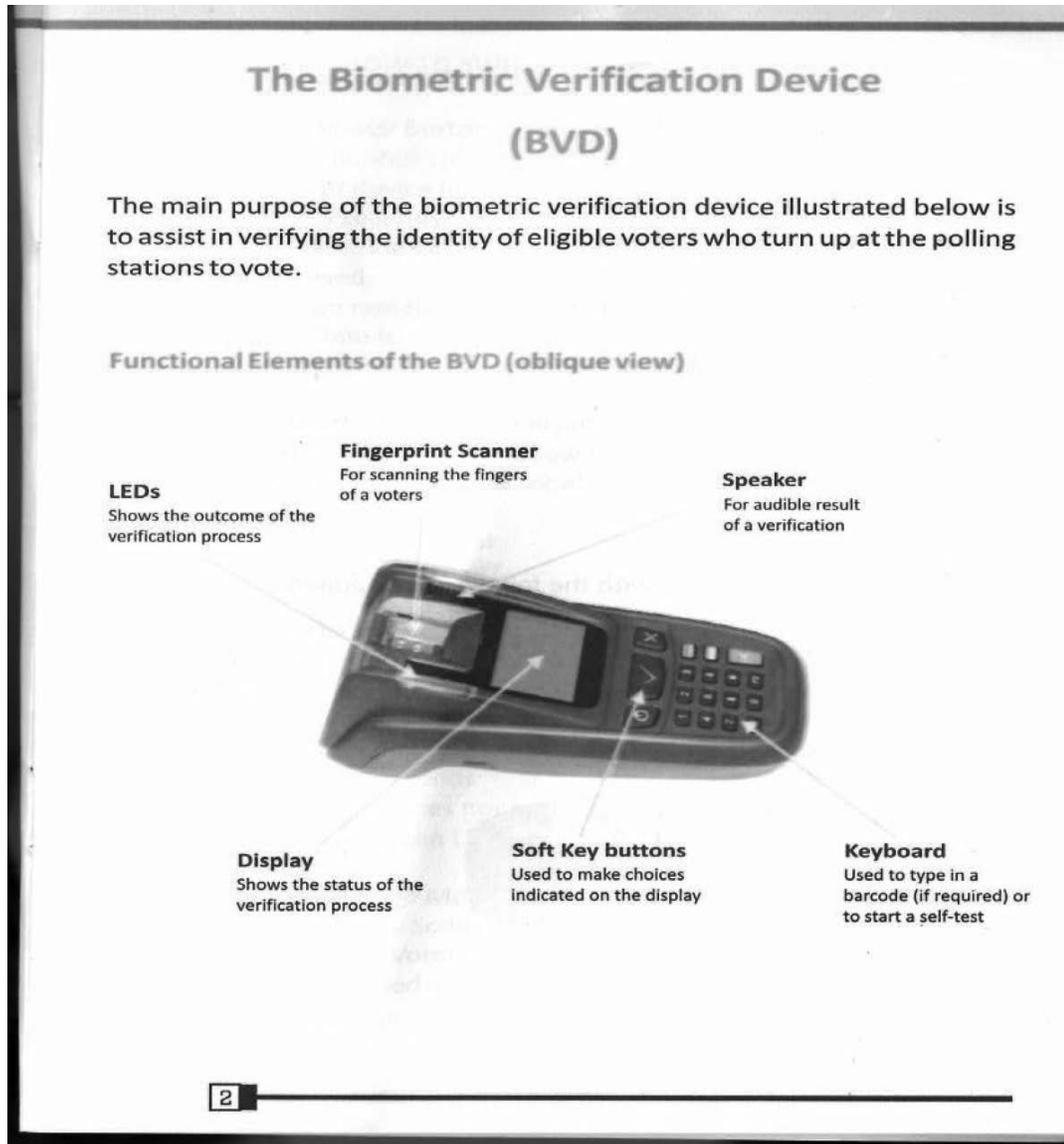
Figure 4.1: Functional elements of the biometric device.<sup>5</sup>
