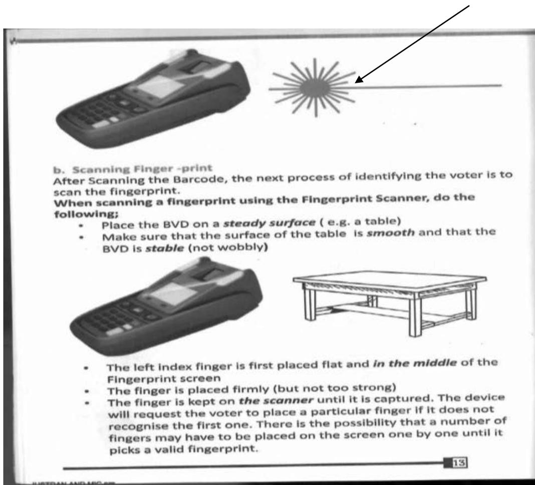
Figure 4.5: Instructions on how device should be positioned before use.<sup>9</sup>
