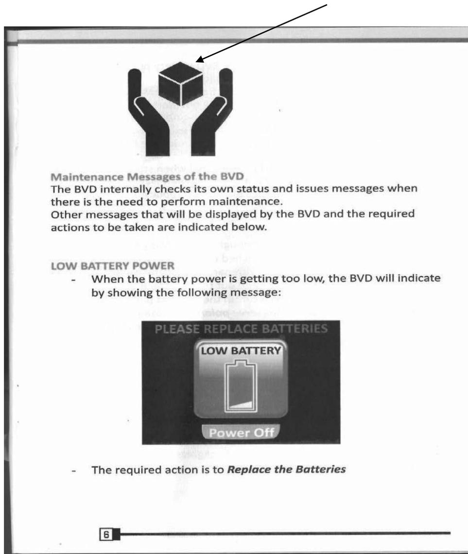
Figure 4.4: Message indicating when to replace batteries.<sup>8</sup>
