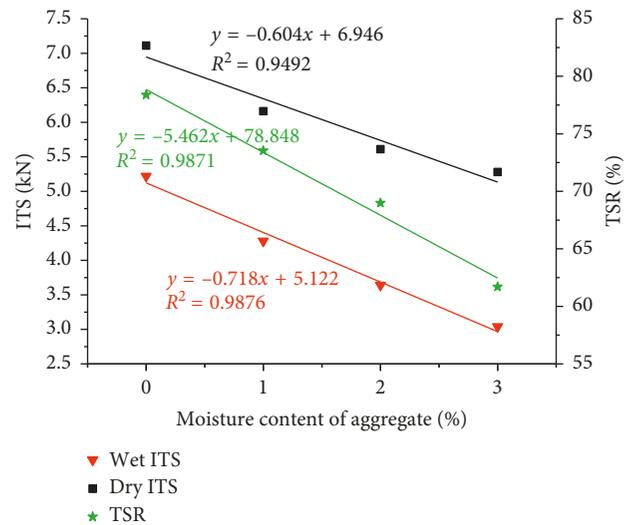
FIGURE 10: ITS/TSR versus moisture contents of an aggregate of the RH-WMA samples.
