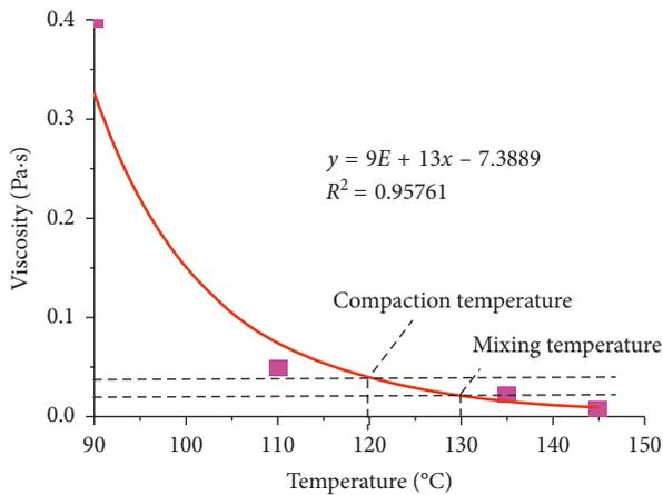
FIGURE 1: Viscosity-temperature curve of the control mix binder.
