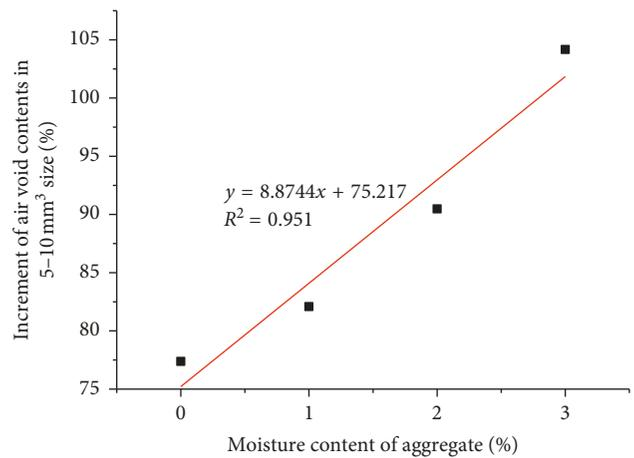
FIGURE 5: Moisture content in aggregates over an increment of air void contents in 5–10 mm<sup>3</sup> size.
