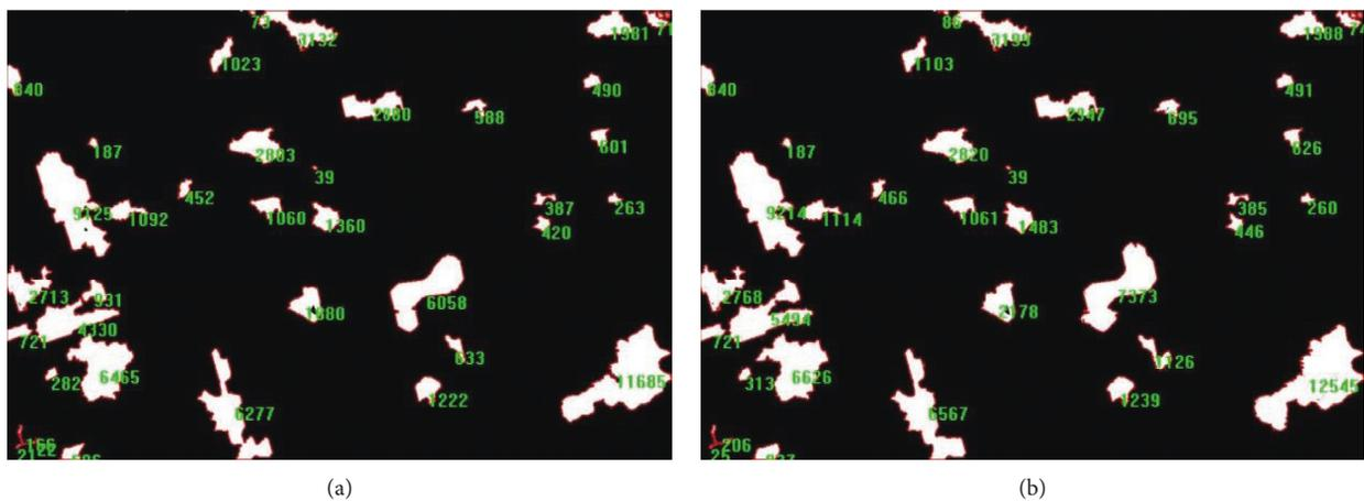
FIGURE 9: Comparisons of air void size of the RH-WMA before and after freeze-thaw cycles. (a) The air void size before freeze-thaw cycles. (b) The air void size after freeze-thaw cycles.
