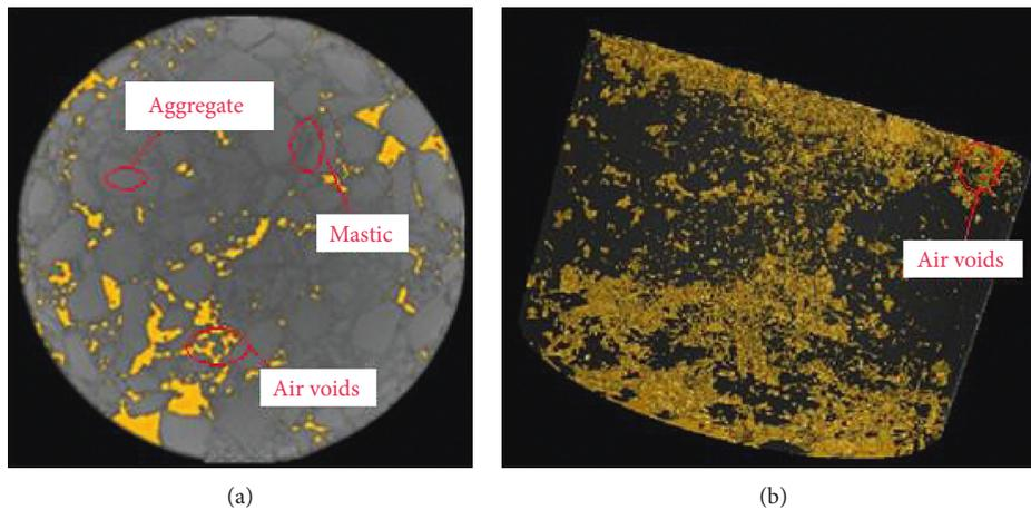
FIGURE 3: 2D and 3D air void segmentation images of the RH-WMA.
