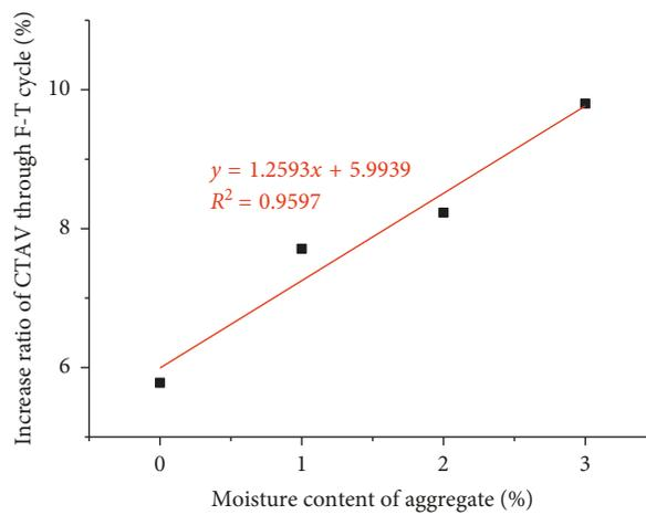
FIGURE 8: Moisture content in aggregates and increase ratio of CTAV through freeze-thaw cycles.
