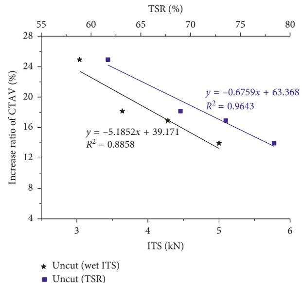
FIGURE 11: ITS/TSR versus increase ratios of CTAV of the RH-WMA.
