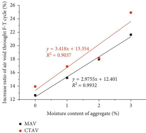
FIGURE 6: Moisture content in aggregates over increase ratio of air voids through freeze-thaw cycles.
