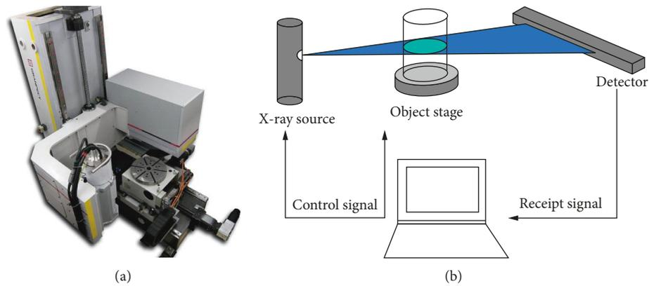
FIGURE 2: The schematic diagram of the industrial computed tomography (CT) system.
