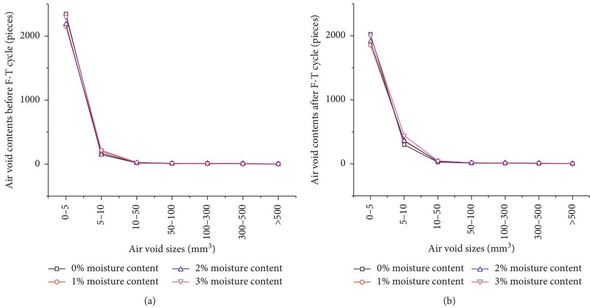
FIGURE 4: Air void contents and their sizes of the RH-WMA through freeze-thaw cycles.
